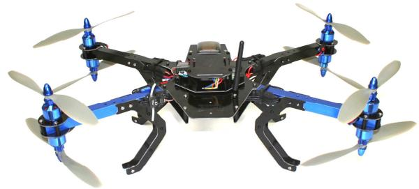
*Fig. 1. 3DR X8 quadcopter with contra-rotating propellers
