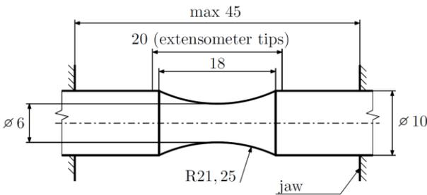
**Fig. 2.** Hourglass specimen
