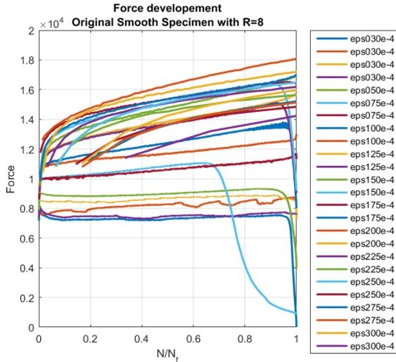
**Fig. 1.** Force progress during fatigue life for original smooth bar specimen. See no-cyclic softening in the end of the fatigue life for most of specimens.
