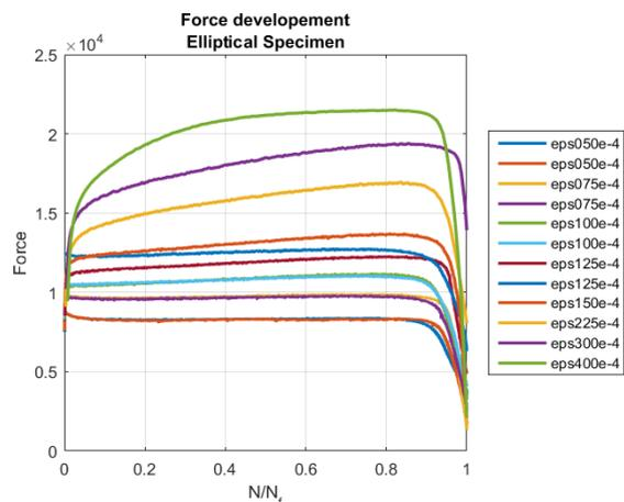
Fig. 7. Force progress during fatigue life for elliptical geometry specimen
