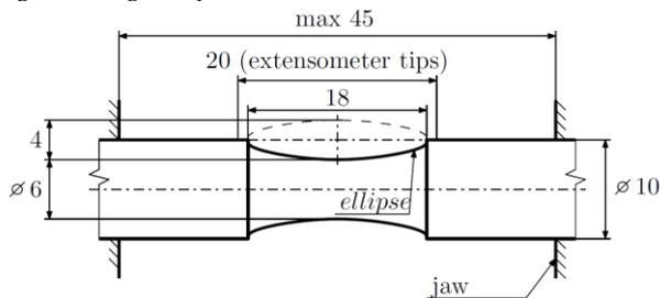
**Fig. 3.** Elliptical geometry specimen
