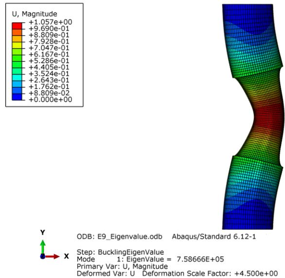
**Fig. 4.** Geometrical imperfection (scaled)
