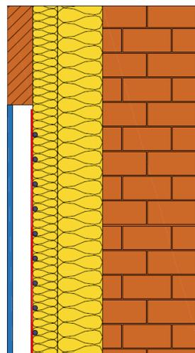
Fig. 1 – Schematic drawing of building integrated solar thermal collector.
