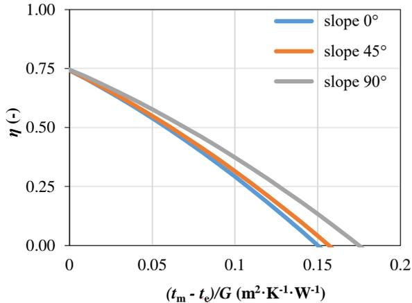
Fig. 2 – Solar collector efficiency curves for different slope angles obtained experimentally.
