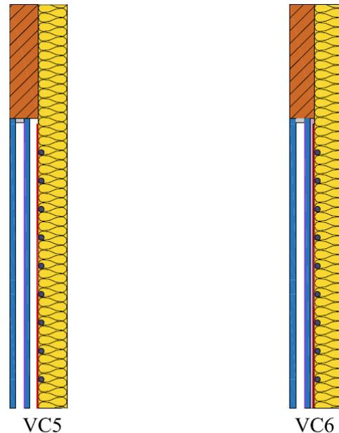
Fig. 6 – Façade collector alternatives with double glazing.
