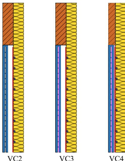
Fig. 5 – Façade collector alternatives with vacuum glazing.
