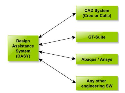
Fig. 3. Design Assistance System (DASY) and connections with different types of software
