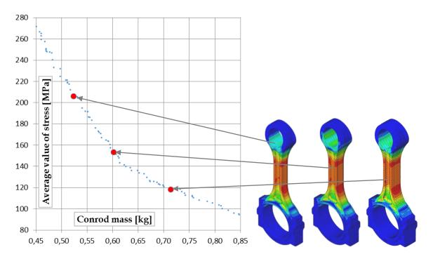
Fig. 6. The output from the design optimization process - Pareto set and different connecting rod design according to the selected design-point.
