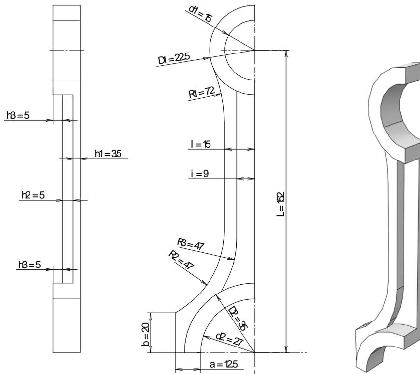
*Fig. 5. A simplified model of the connecting rod with parameters for simulation in Abaqus system.*
