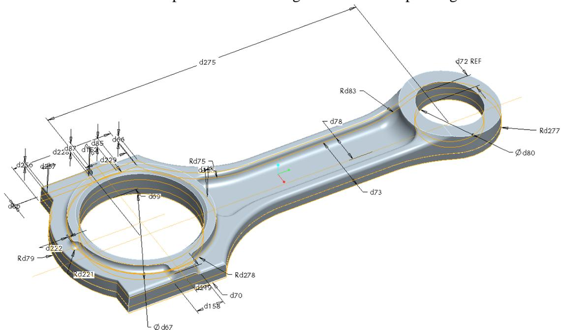
*Fig. 1. A 3D CAD model of a connecting rod with the parameters (dimensions)*
