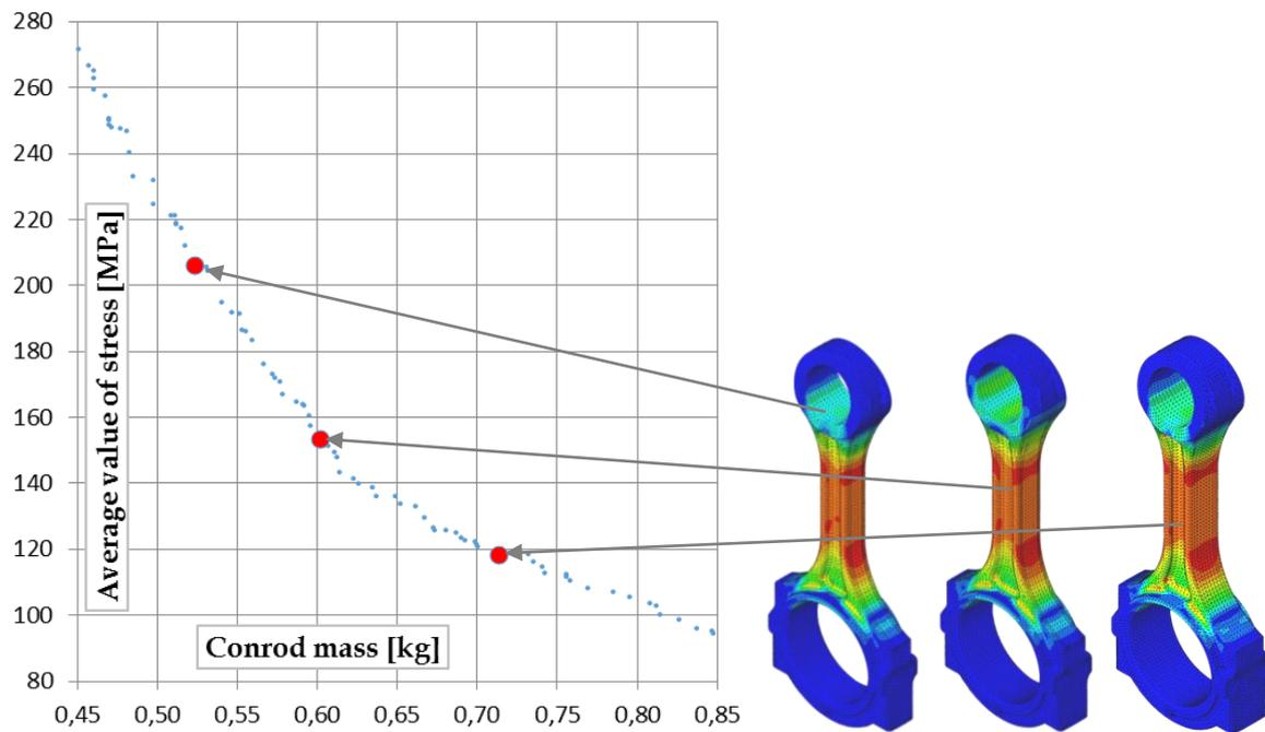
*Fig. 6. The output from the design optimization process - Pareto set and different connecting rod design according to the selected design-point.*
