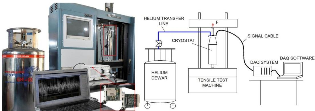
**Fig. 3.** Experimental set-up for tensile test at cryogenic temperature
