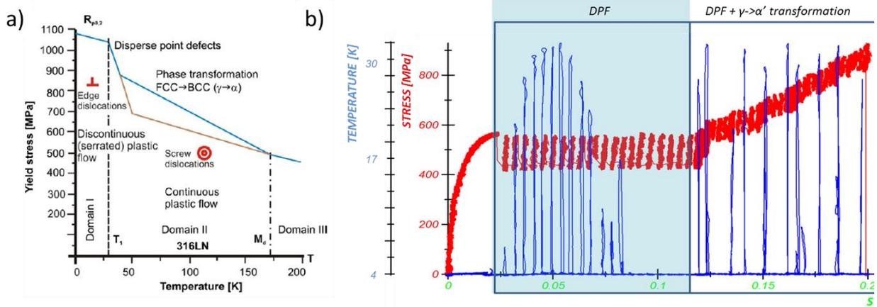
**Fig. 1.** (a) Yield point against temperature for austenitic stainless steel [1] (b) Stress-strain and temperature-strain curves obtained for uniaxial tensile test at liquid helium temperature (4,2K) for austenitic steel specimen (304)
