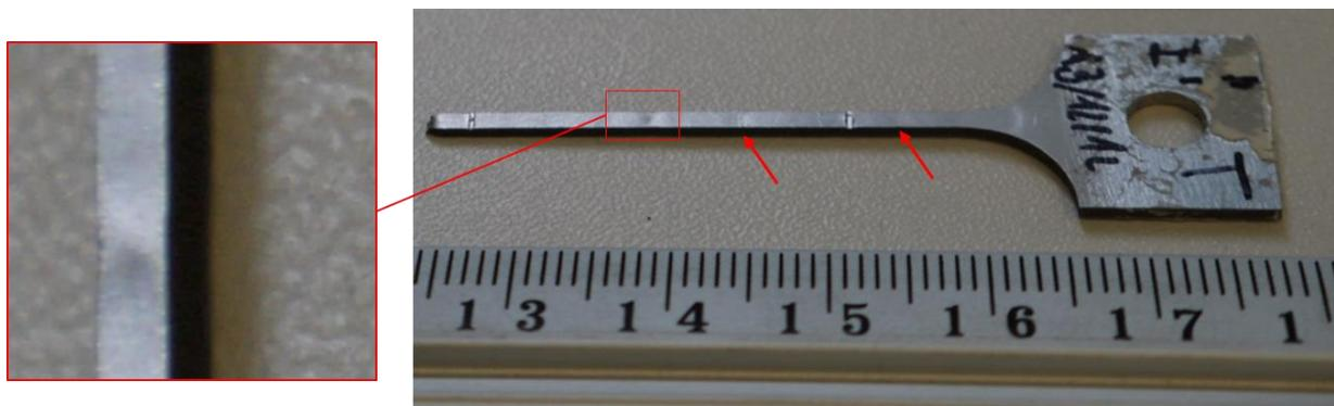
**Fig. 6.** Multi-necking effect during uniaxial tensile test of austenitic steel specimen at liquid helium temperature
