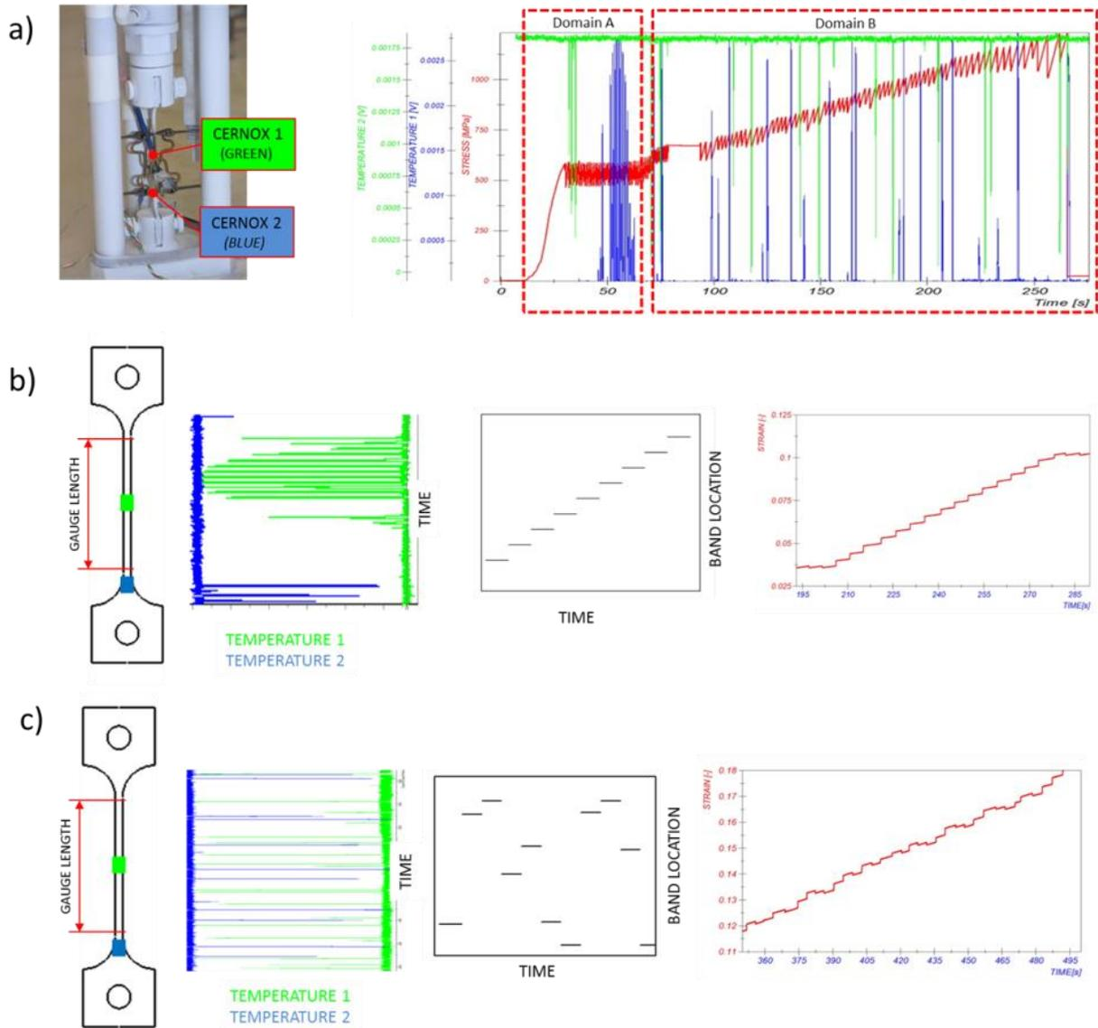
**Fig. 5.** (a) Stress (red), temperature 1 (green), and temperature 2 (blue) in time domain for 304 steel specimen during strain-controlled tensile test at 4,2K, (b) schematic of slip band motion and orientation for domain A (DPF), (c) schematic of slip band motion and orientation for domain B (DPF +  $\gamma \rightarrow \alpha'$  transformation).
