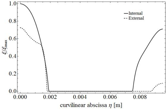
Fig. 4. Distribution of martensitic phase along the curvilinear abscissa  $\eta$  (external and internal side, see Fig.3.)
