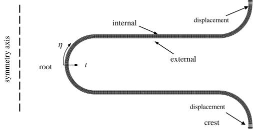
Fig. 3. Boundary conditions and finite element mesh of expansion bellows
