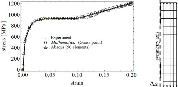
Fig. 1. Stress-strain curve for 316L stainless steel at 4.2K (left), model implemented in Abaqus/Explicit (right)
