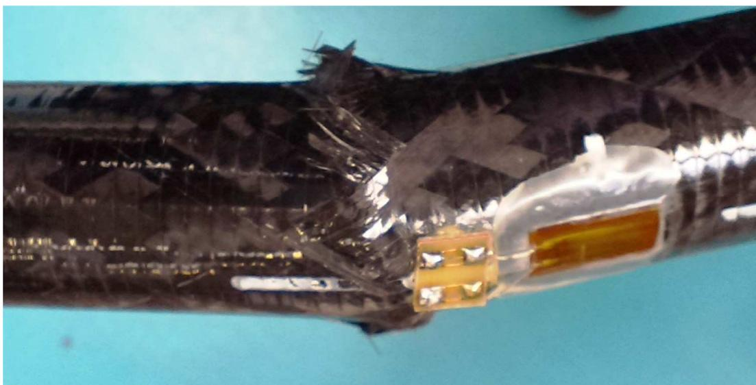
*Figure 6. Broken tube with damping layer*
