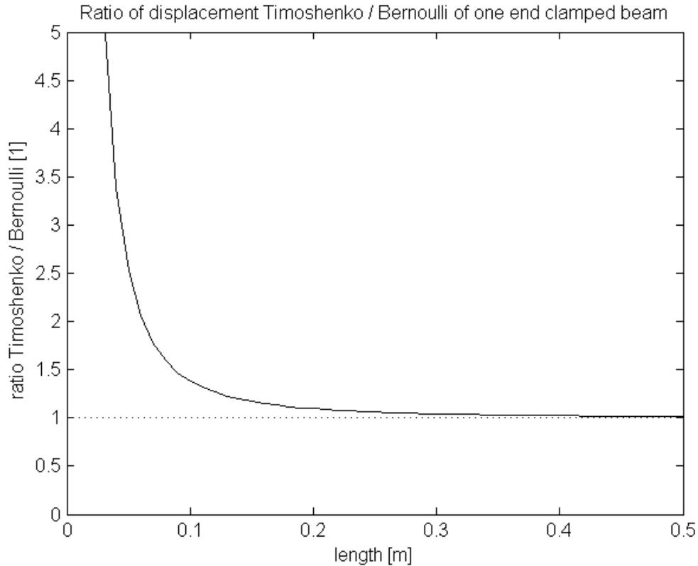
**Figure 3.** Ratio of displacement Timoshenko / Bernoulli of one end clamped beam
