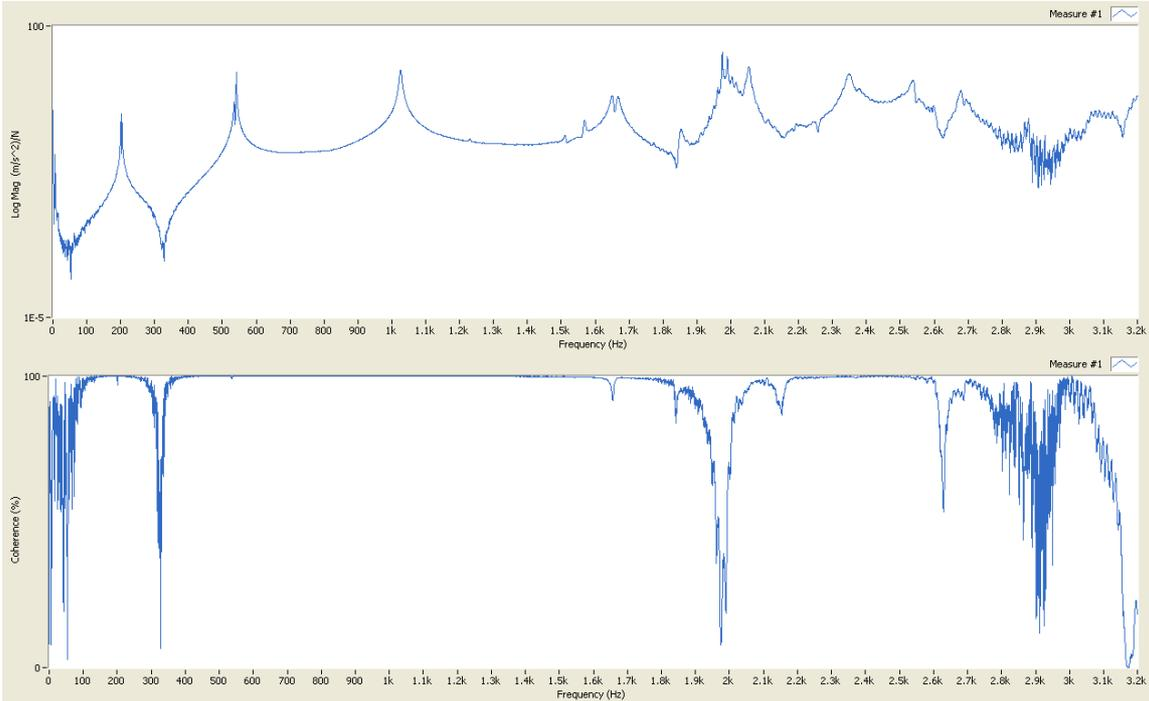
**Figure 8.** Example of Transfer function and Coherence for one measuring point
