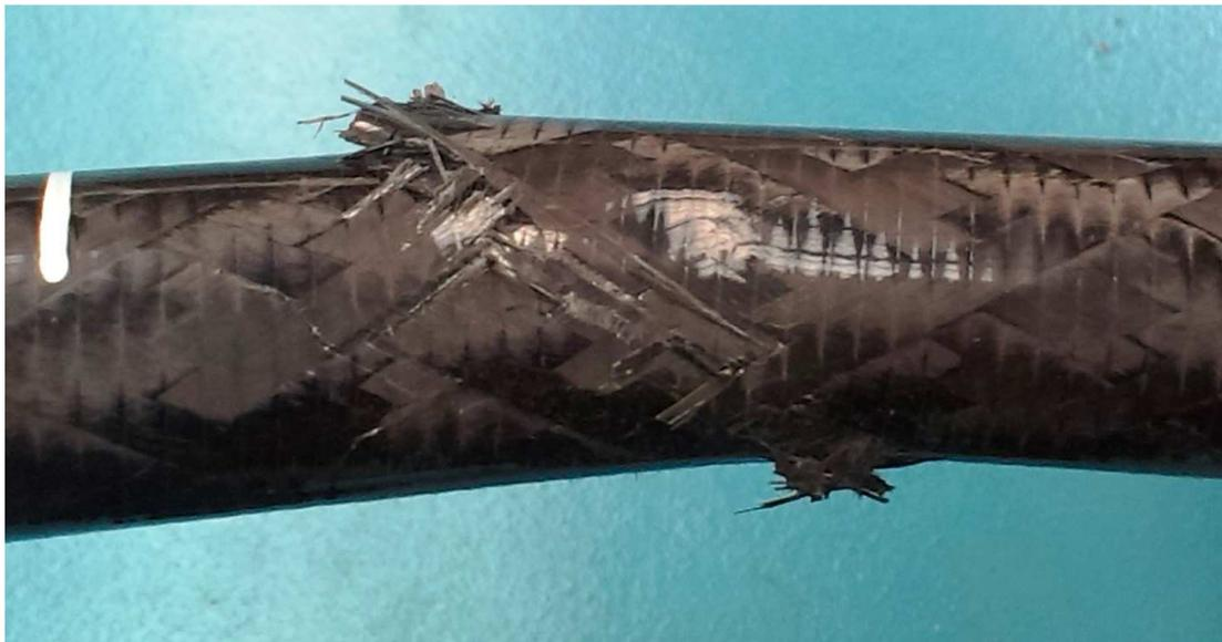
*Figure 5. Broken tube without damping layer*
