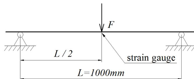
**Figure 4.** Bending 3-point test
