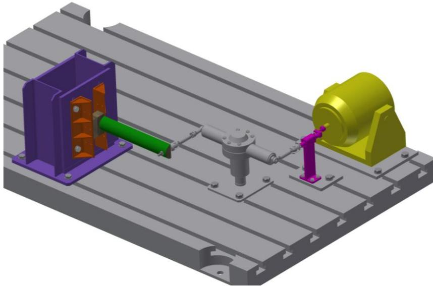
**Figure 15.** The assembly of bending testing machine. The main aim of this testing machine is to verify FE calculations.
