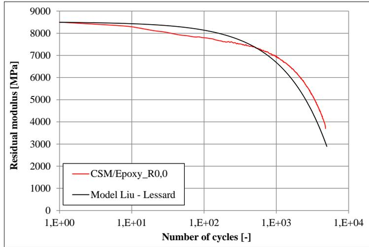
**Figure 7.** Residual stiffness curve of CSM/Epoxy composite measured during 1D tension fatigue test and the curve, which is representing identified degradation model Liu – Lessard.
