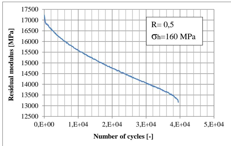
**Figure 1.** Residual stiffness curve of glass/epoxy laminate -  $[(0/90)_8]$ . Reinforcement was realized by fabric  $280 \text{ g/m}^2$  with plain weave embedded in epoxy resin [8].
