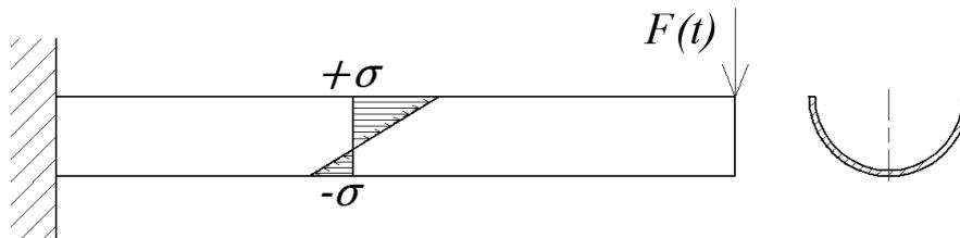
**Figure 8.** Scheme of fixed beam, which was modelled using FEM in order to test degradation models.
