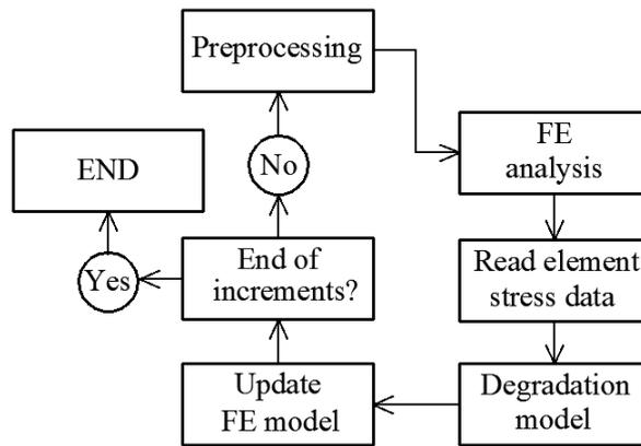
**Figure 5.** Block scheme of computational algorithm for calculations of stiffness reduction in in-plane isotropic laminates.
