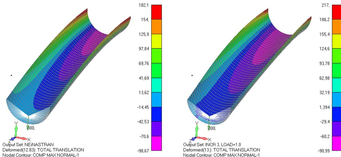
**Figure 4.** The comparison of the distribution of stress  $\sigma_L$  from linear and non-linear analysis of thin-walled structure. Deformation scale factor is 5.
