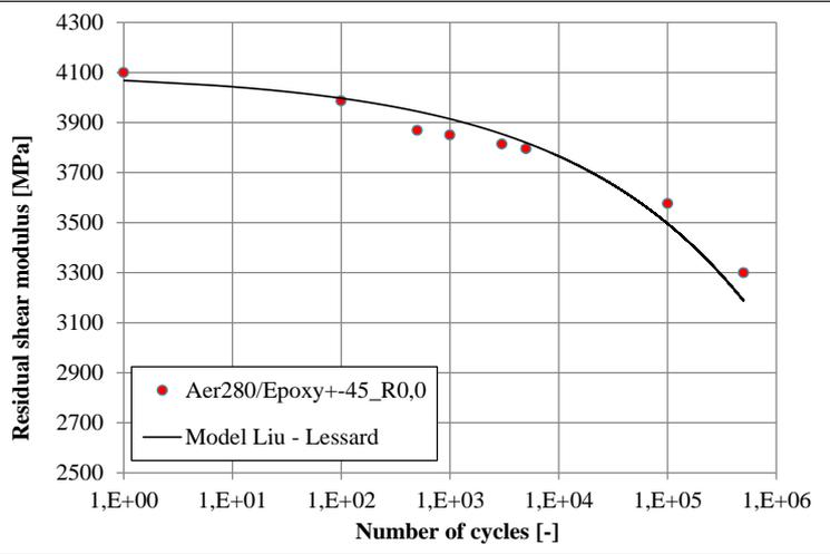
**Figure 12.** Residual shear modulus  $G_{LT}$  of laminate, which was reinforced by balanced fabric  $[(0/90)_3]$  and identified model Liu – Lessard.
