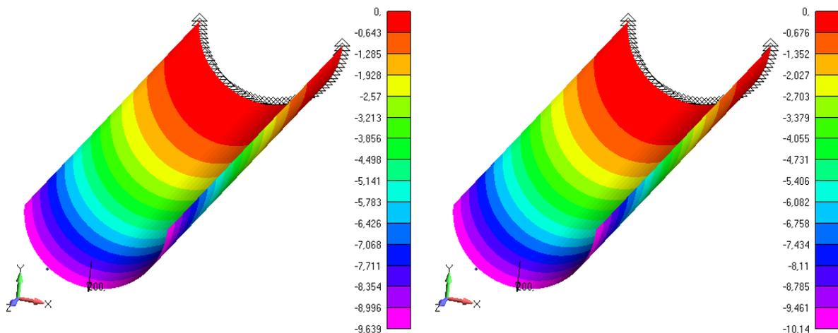
**Figure 10.** The comparison of displacements in the direction of loading force (y direction). Displacements increased by 0,5 mm.
