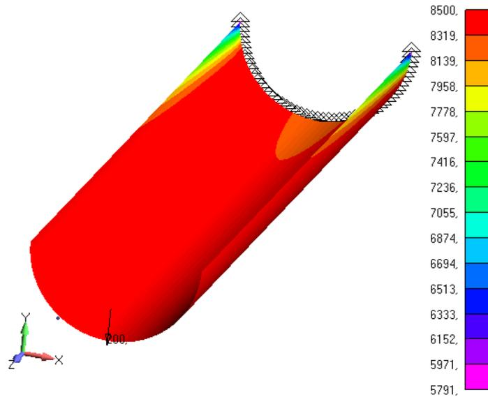
**Figure 9.** The distribution of residual modulus after 5000 cycles. A virgin modulus value was set to 8500 MPa and the lowest value of residual modulus is 5791 MPa.
