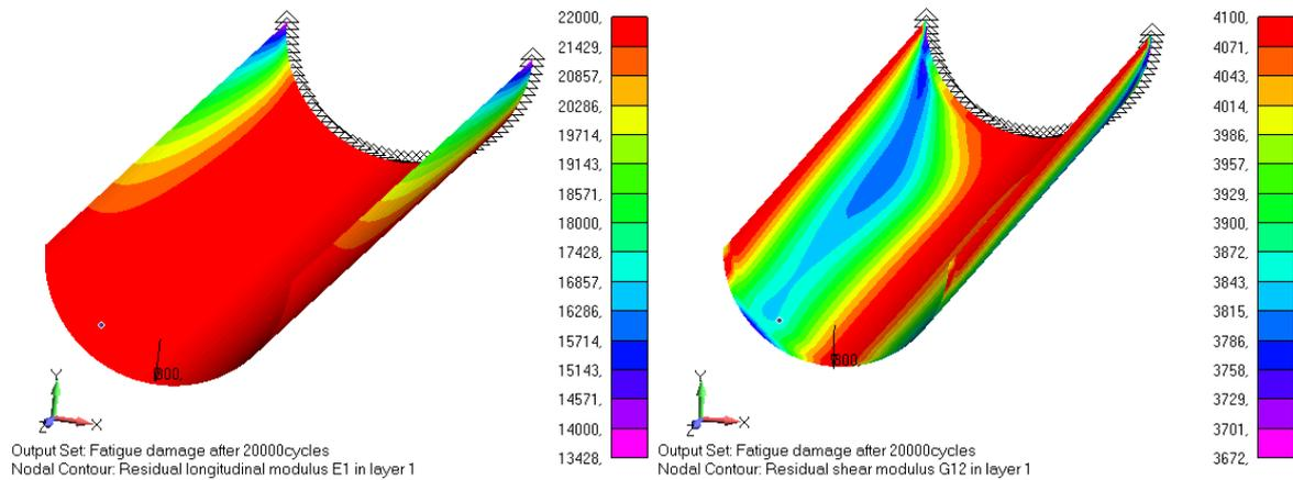
**Figure 13.** The results of FE calculations of residual moduli  $E_L$  (on the left) and  $G_{LT}$  (on the right) in the first layer after  $2.10^4$  cycles.
