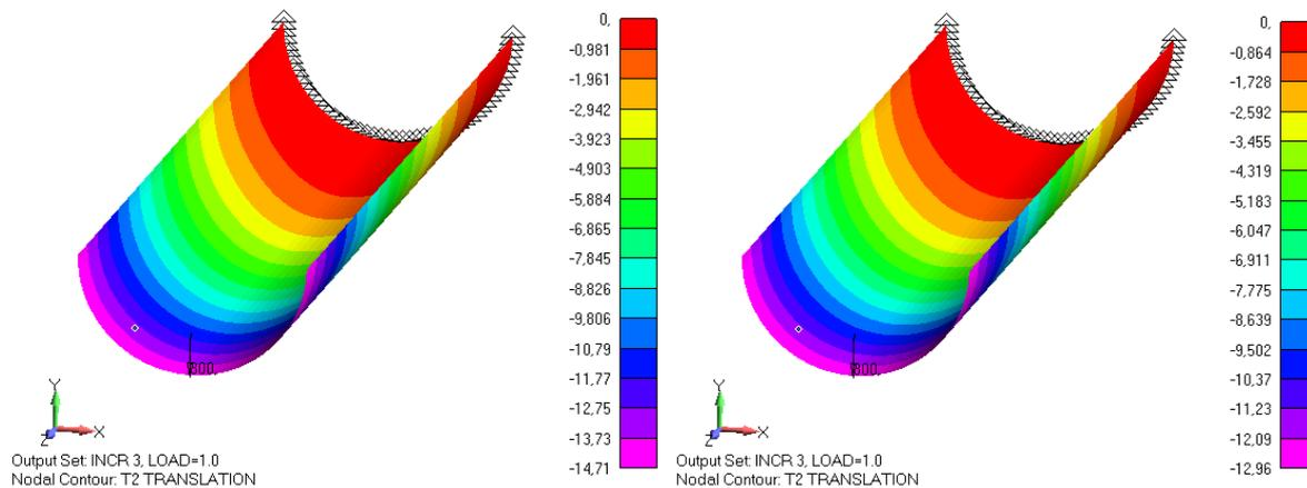
**Figure 14.** The comparison of displacements of virgin structure (on the right) and after  $2.10^4$  cycles (on the left). The increase of displacements is 1,75 mm.
