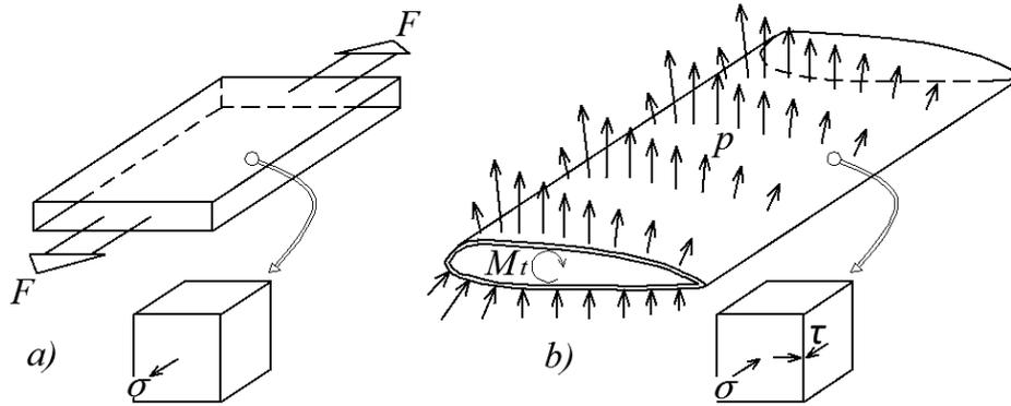
**Figure 2.** Mechanical model of unidirectional tensile test – part a) and a mechanical model of thin walled composite wing, which is loaded with a pressure field and torque – part b). The difference between stress states of both loading modes is obvious in shown infinitesimal volumes.
