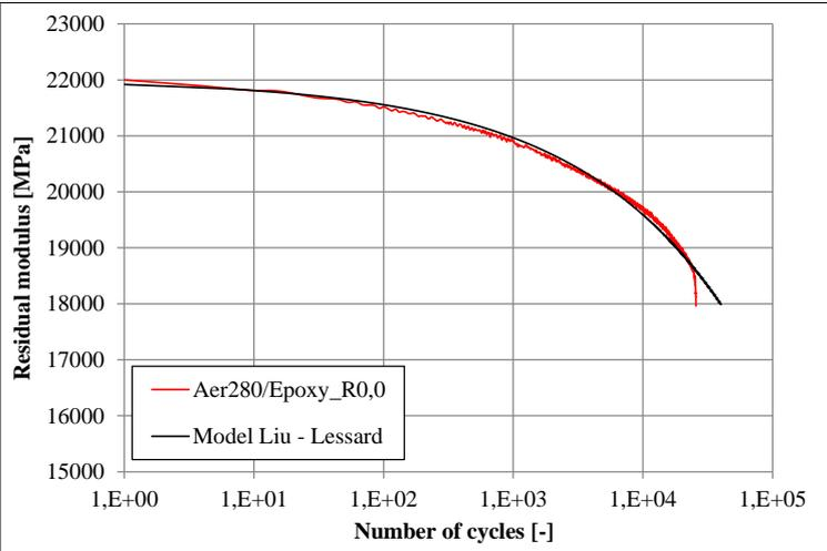
**Figure 11.** Residual modulus  $E_L$  curve of laminate, which was reinforced by balanced fabric  $[(0/90)_3]$  and identified model Liu – Lessard.
