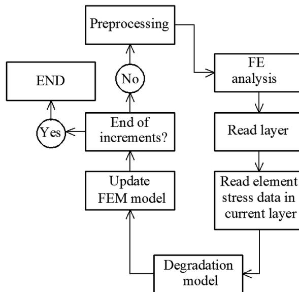
**Figure 6.** Block scheme of computational algorithm for calculations of stiffness reduction of orthotropic laminates.
