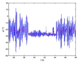
Fig. 22: Relative rotation of the gearbox to the asynchronous motor round the axis z for common drive regime, section with ess curve
