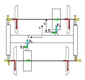
Fig. 3: Parasitic lateral forces, [3]
