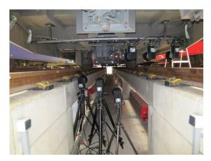
Fig. 9: Stationary and moving system of cameras
