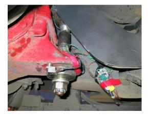
Fig. 11: Mounted and connected gearbox hinge
