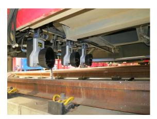
Fig. 10: Moving system of cameras mounted to the holder
