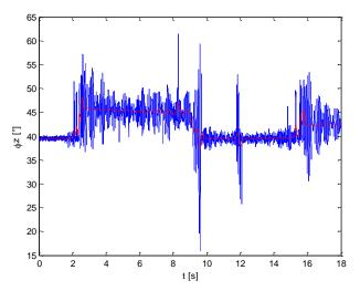
Fig. 17: Relative rotation of the gearbox to the asynchronous motor round the axis z for acceleration regime
