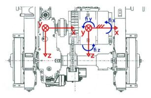
*Fig. 8: Cartesian coordinate systems of the gearbox and the asynchronous motor*
