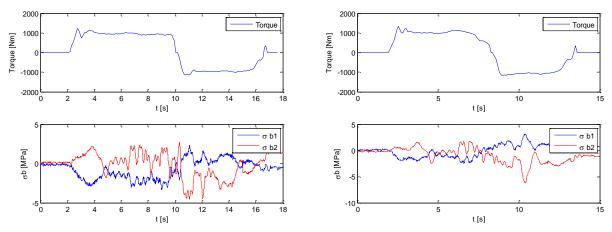
Fig. 14: Torque of two asynchronous motors and bending stress in two perpendicular planes for acceleration (left) and deceleration (right)
