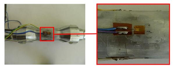
Fig. 5: Strain gauges installed on the hinge
