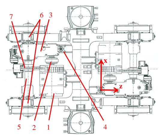
*Fig. 1:* Schema of the tram drive placed on the chassis – 1-Asynchronous motor, 2-Claw coupling, 3-Gearbox, 4-Gearbox hinge, 5-Mounted wheels, 6-Bearing units, 7-Disc brake
