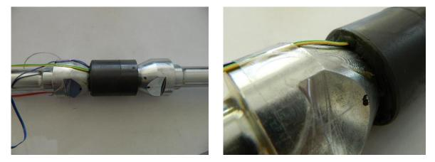
Fig. 6: Protective cover of the hinge with the strain gauges
