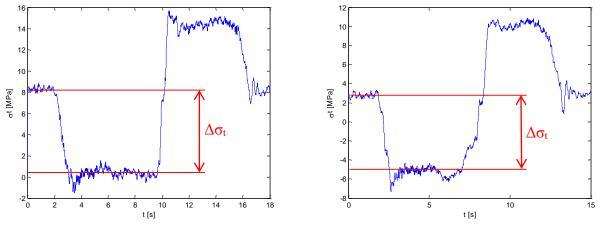
Fig. 16: Tensile stress in the hinge for acceleration (left) and deceleration (right)
