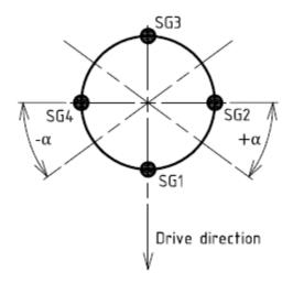
Fig. 4: Measuring arrangement of the strain gauges
