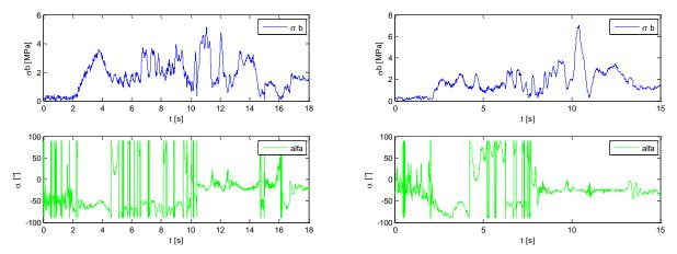
Fig. 15: Resultant of bending stress and its orientation for acceleration (left) and deceleration (right)
