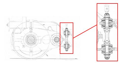
Fig. 2: Gearbox hinge design, [3]
