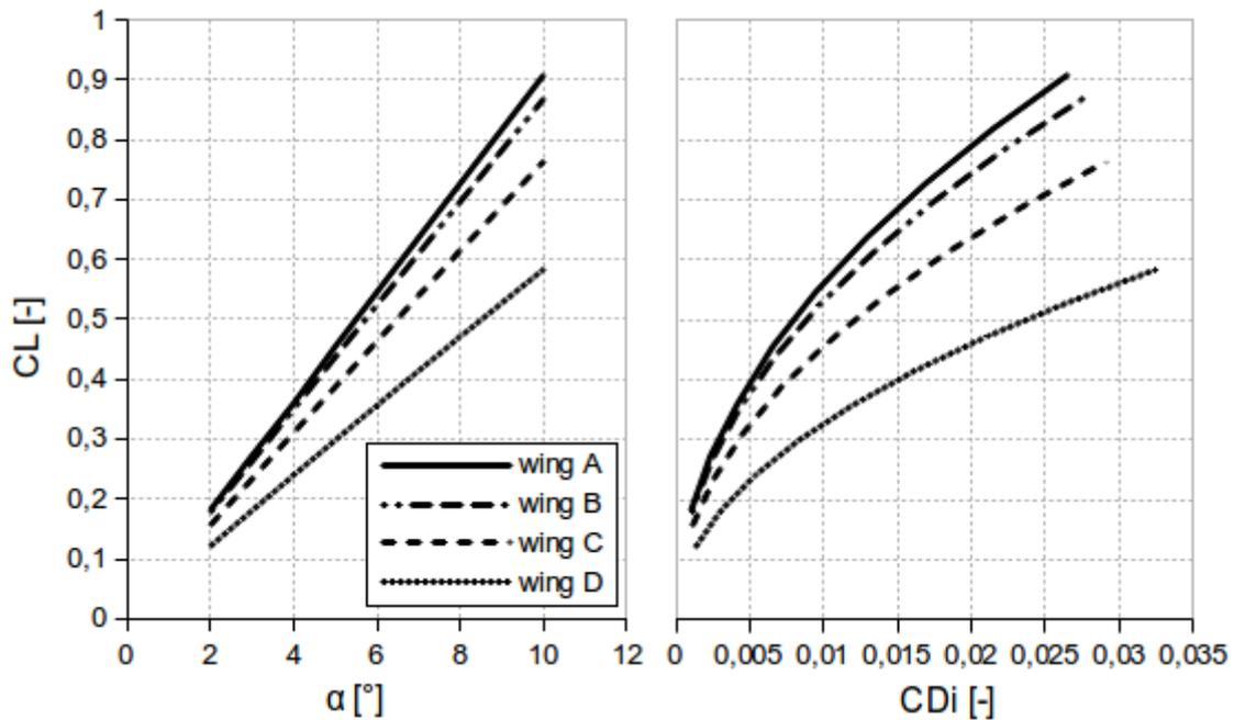
Fig. 9. Lift curve and drag polar of chambered wings
