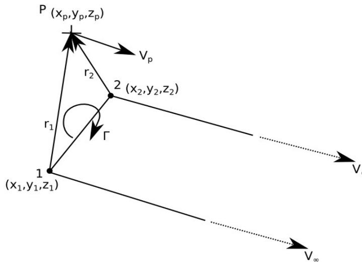
**Fig. 3.** Induced velocity by horseshoe element
