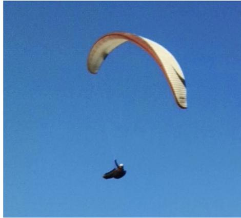
**Fig. 6.** Typical paraglider having spanwise chamber
