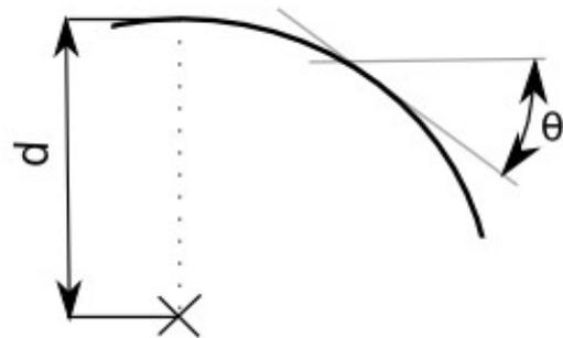
**Fig. 7.** Geometry of circular arc wings
