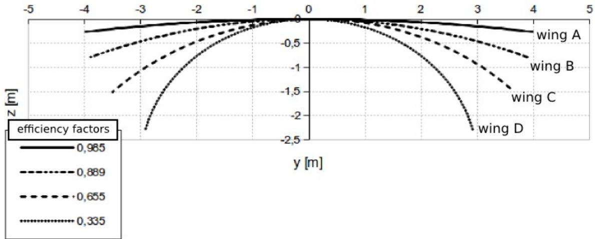
Fig. 8. Circular arc lifting line and their efficiency factors
