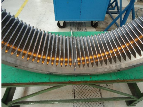
Fig. 1 Ring gear with strain gauges and epoxide layer
