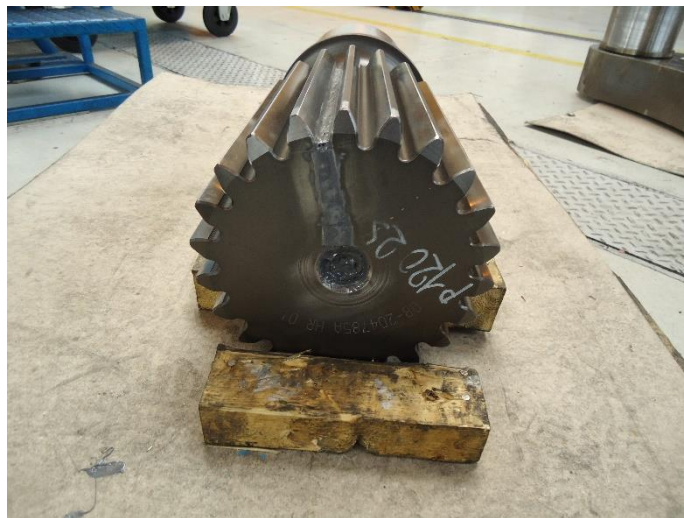
Fig. 2 Pinion with strain gauges and epoxide layer
