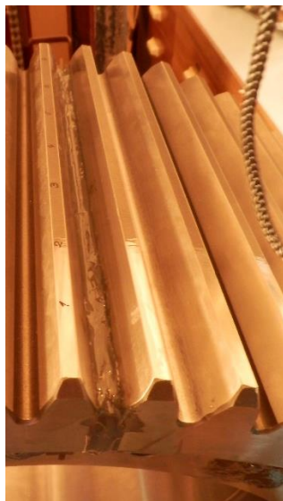
Fig. 3 Planet gear with strain gauges and epoxide layer
