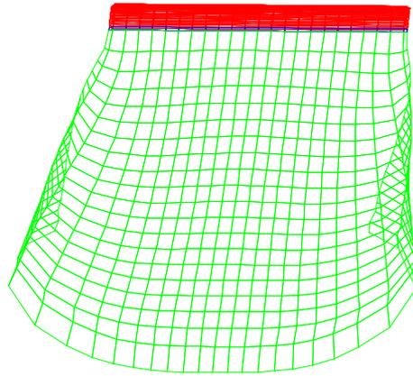
**Fig.5** – Wake formation after 20 iterations behind the NACA 4412 airfoil wing.
