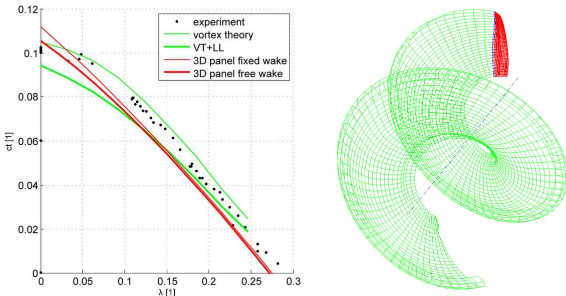
**Fig.6** – Left: Comparison of thrust according to simulation and experiment. Right: Wake formation behind single rotating blade
