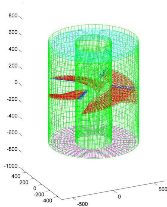
*Fig.7 – Mesh of the third test case – Kaplan turbine in an internal domain*
