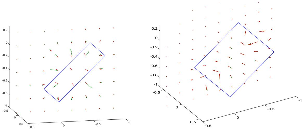
**Fig.2** – Flow field around panels. Left: Source panel. Green color represents velocity by point source in the middle of panel, red color represents velocity induced by continuous distribution of source across the panel. Right: Vortex ring panel and its induced velocity .
