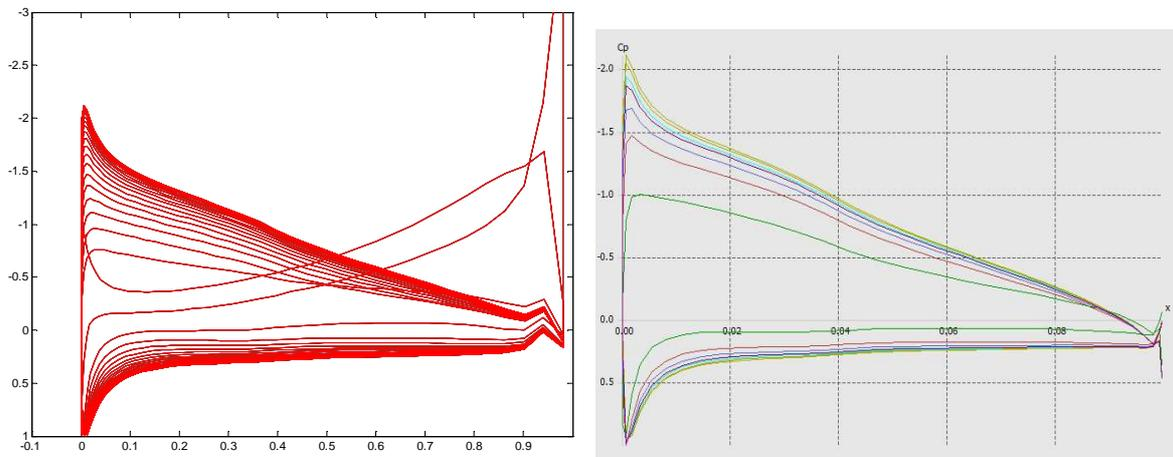
**Fig.4** – Pressure coefficient at different cross sections of NACA 4412 airfoil finite wing under  $10^\circ$  angle of attack. Left: Author's panel code, Right: XFLR5 software
