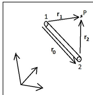
**Fig.1** – Vortex filament segment and its influence on point P.
