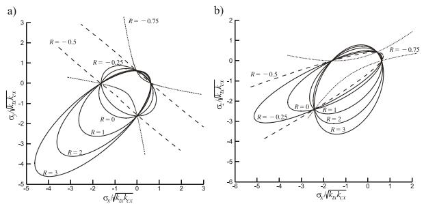
**Fig. 1.** Convexity loss of tetragonal Tsai-Wu criterion in case of high orthotropy degree for traverse isotropy: a) plane of transverse isotropy ( $\sigma_x$ ,  $\sigma_y$ ), b) plane of orthotropy ( $\sigma_x$ ,  $\sigma_z$ ).
