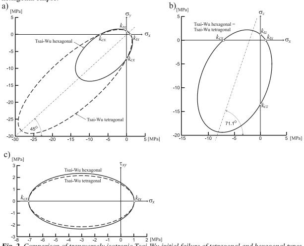
**Fig. 2.** Comparison of transversely isotropic Tsai-Wu initial failure of tetragonal and hexagonal types for columnar ice in case of: a) plane of traverse isotropy  $(\sigma_x, \sigma_y)$ , b) plane of orthotropy  $(\sigma_x, \sigma_z)$ , c) shear plane  $(\sigma_x, \tau_{xy})$ .
