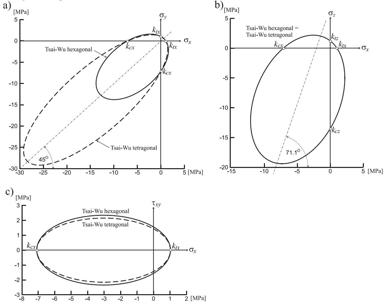
**Fig. 2.** Comparison of transversely isotropic Tsai-Wu initial failure of tetragonal and hexagonal types for columnar ice in case of: a) plane of traverse isotropy  $(\sigma_x, \sigma_y)$ , b) plane of orthotropy  $(\sigma_x, \sigma_z)$ , c) shear plane  $(\sigma_x, \tau_{xy})$ .
