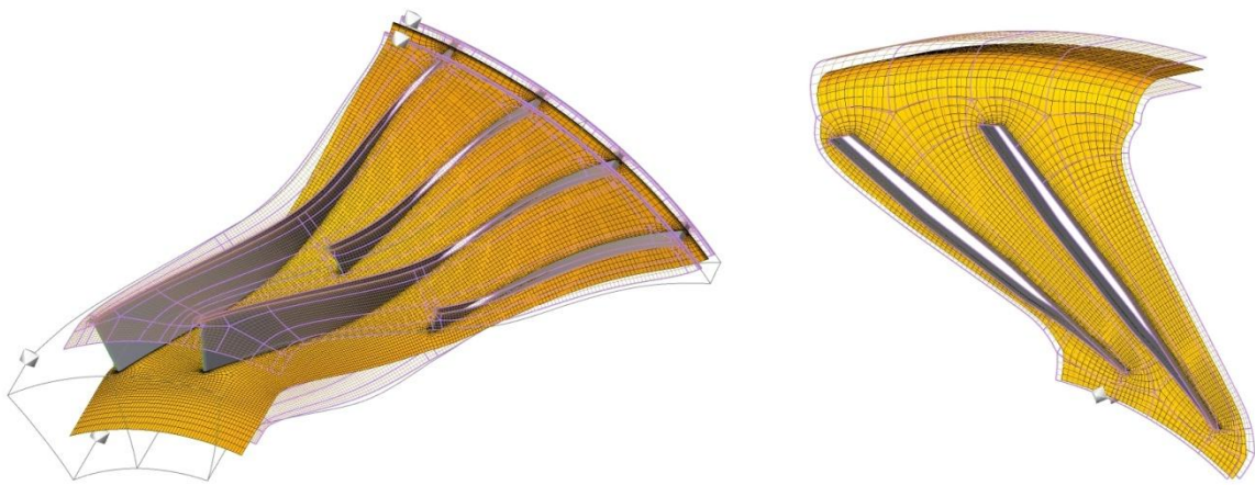
Fig. 7. Left, the impeller computational mesh. Right, the diffuser mesh
