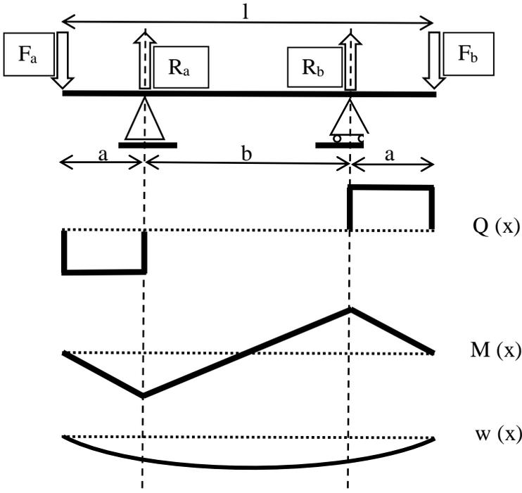
Figure 2. Overhanging beam representing static load acting on the axle with subjected shear force, bending moment and deflection.
