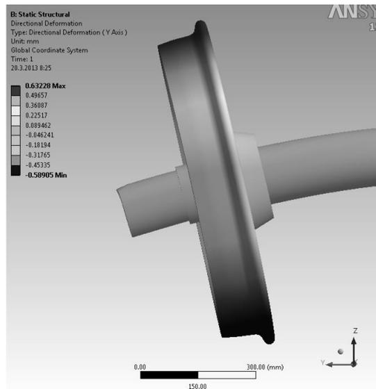
Figure 5 Example of Ansys graphic interpretation of deformation results on the wheel
