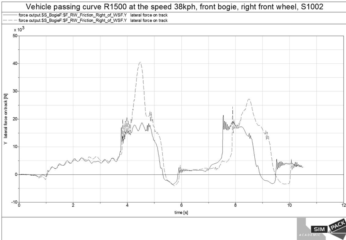
Figure 8. - Lateral force acting in the tread contact between right front wheel of front bogie and rail (rail profile is UIC 60, its cant 1:40 and gauge 1435mm). Vehicle is passing the curve R1500 at the speed of 38kph. The UIC-S1002 wheel profile was used.
