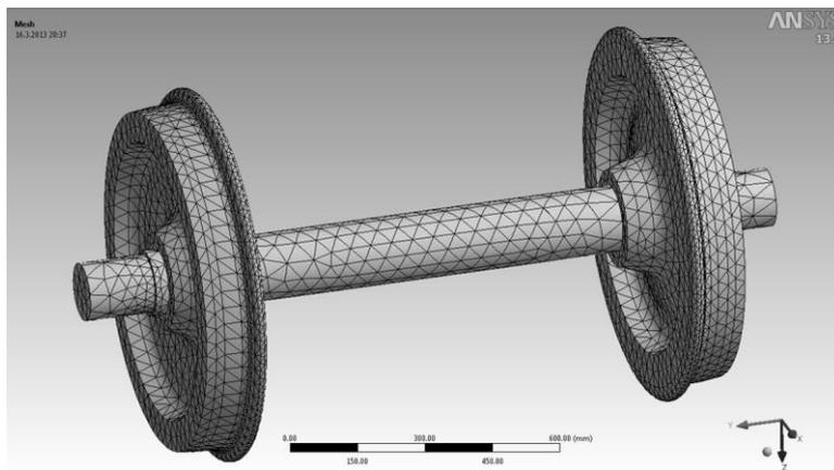
Figure 3 Model of wheel set in Ansys and its mesh.
