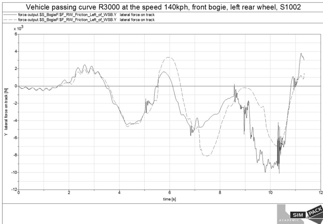
Figure 7. - Lateral force acting in the tread contact between right front wheel of front bogie and rail (rail profile is UIC 60, its cant 1:40 and gauge 1435mm). Vehicle is passing the curve R3000 at the speed of 140kph. The UIC-S1002 wheel profile was used.
