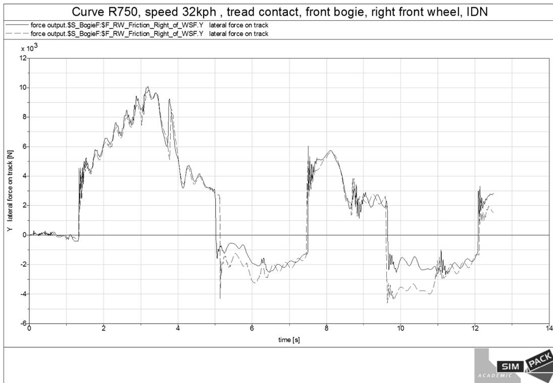
Figure 6. - Course of the lateral force acting in the tread contact between right front wheel of front bogie and rail (rail profile is UIC 54, its cant 1:40 and gauge 1067mm). Vehicle is passing the curve R750 at the speed of 32kph. The conical wheel profile was used.
