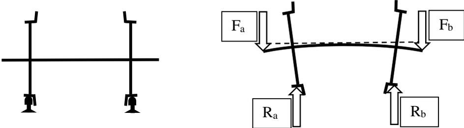
Figure 1. Scheme of wheelset and its expected bending deflection caused by forces  $F_a$  and  $F_b$  – these represent static load
