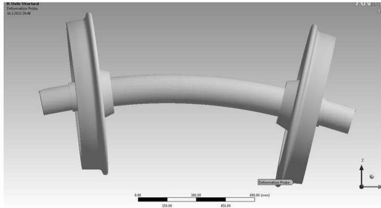
Figure 4 Deformed wheel set calculated by Ansys
