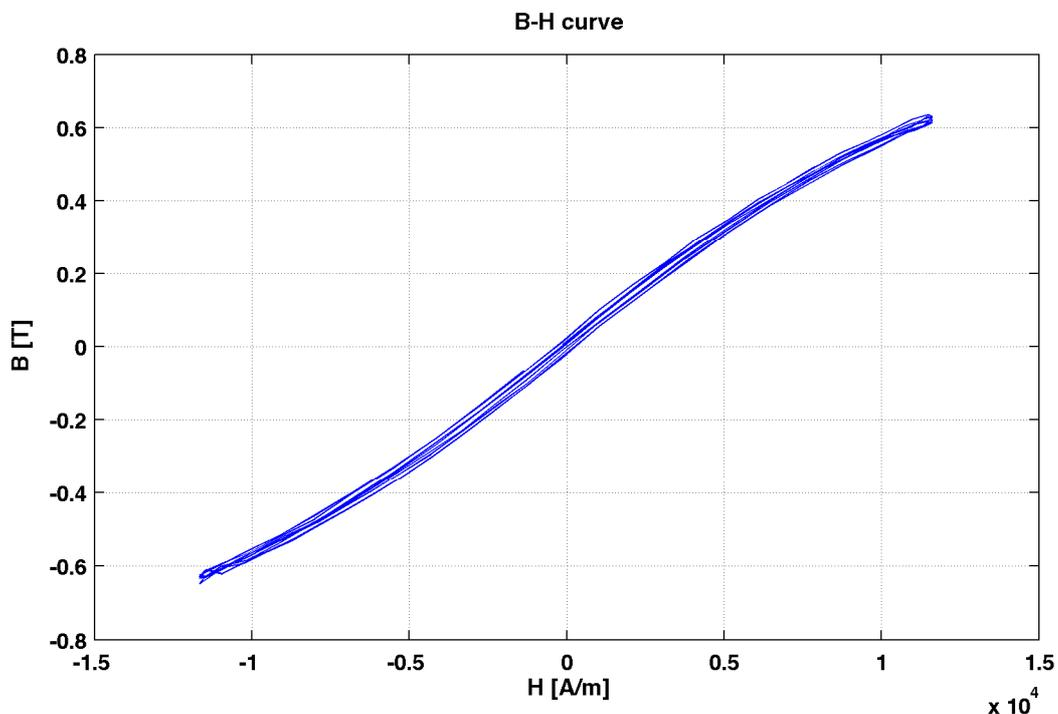
**Fig. 4** Hysteresis loop of the toroidal shape core; applied current 3 A, applied frequency 250 Hz
