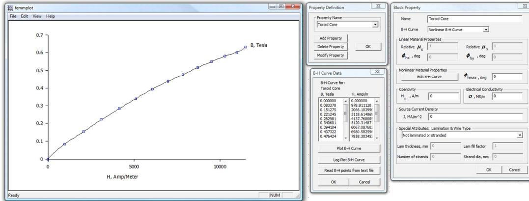
Fig. 6 Inserting data of B-H curve into FEMM software
