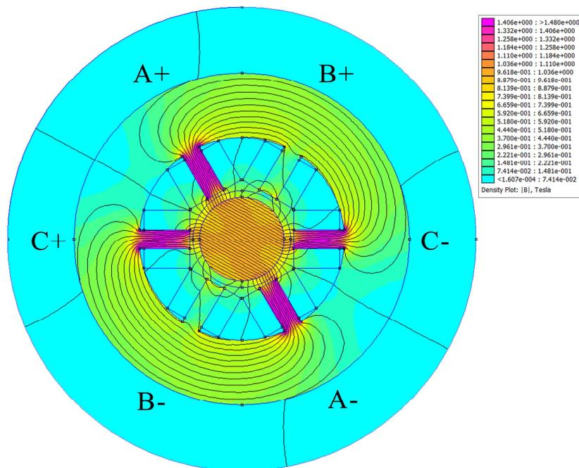
Fig. 7 Result of FEM analysis with one active pole pair B+ and B-; current 3A
