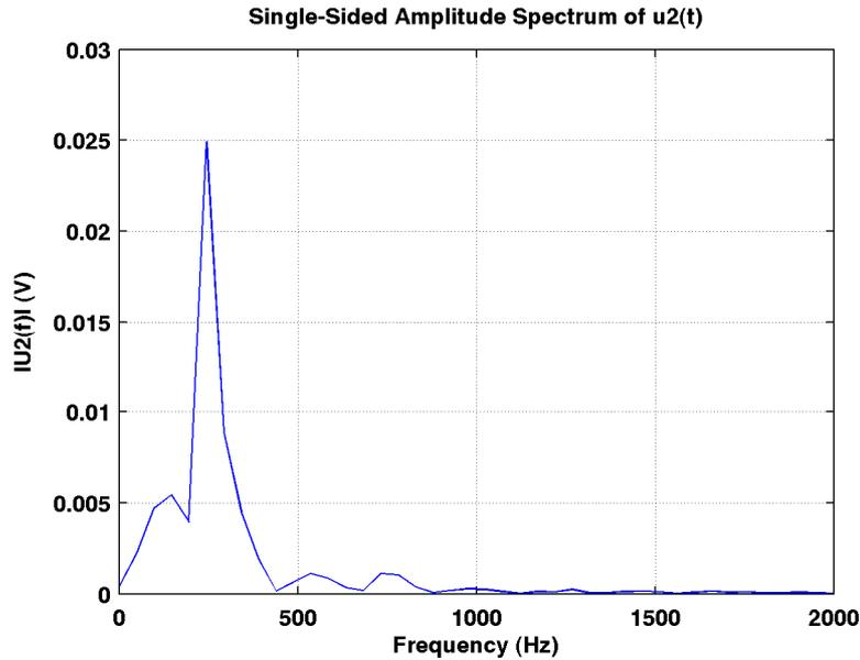
*Fig. 5 Single-sided amplitude spectrum of  $u_2(t)$ ; applied current 3A, applied frequency 250 Hz*
