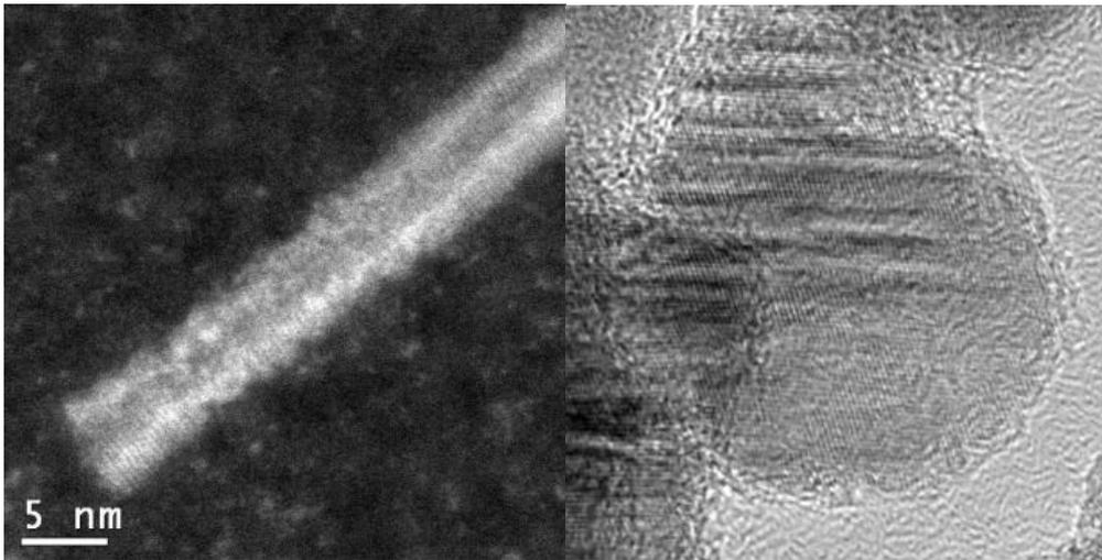
**Figure 1.** (a)  $WO_3$  (gas sensors) (b) ZnS (electronics)
