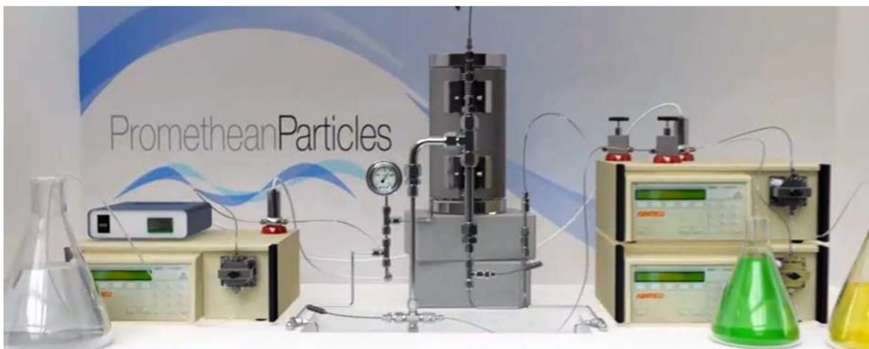
**Figure 3.** The SHYMAN continuous hydrothermal reactor
