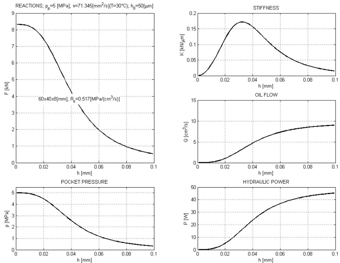
Fig. 5: Characteristics of the hydrostatic system with constant resistance regulation
