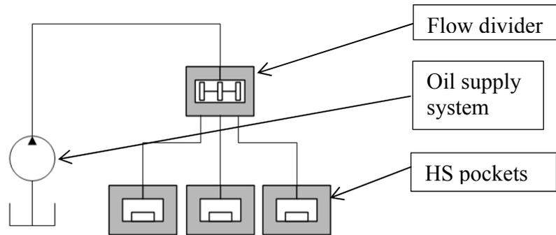
Fig. 3: Connection of the constant flow rate regulation with gear flow divider
