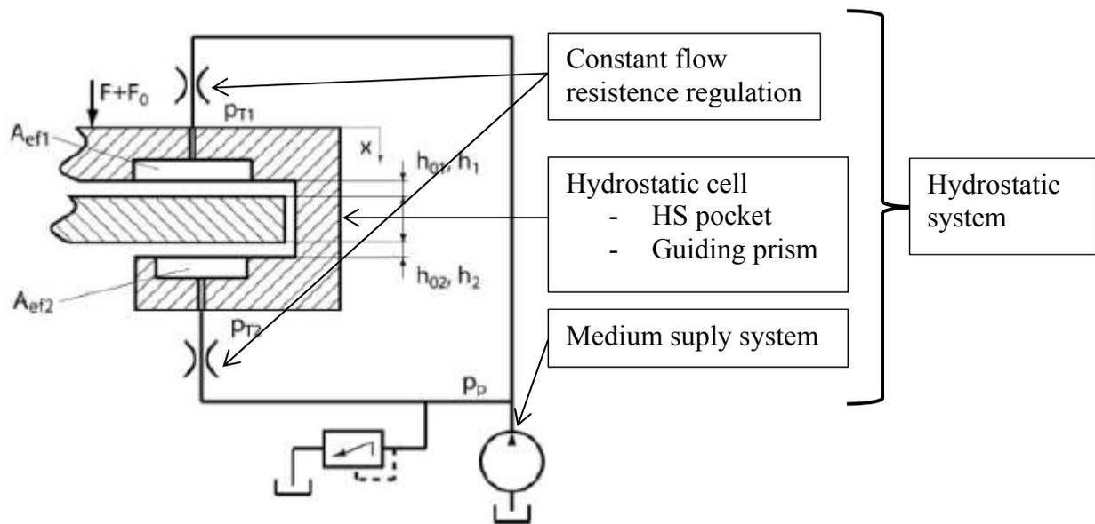
Fig. 1: Components of hydrostatic system
