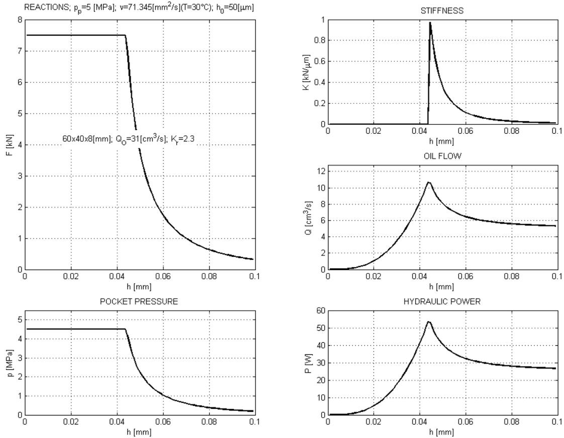
Fig. 6: Characteristics of the hydrostatic system with PM regulator
