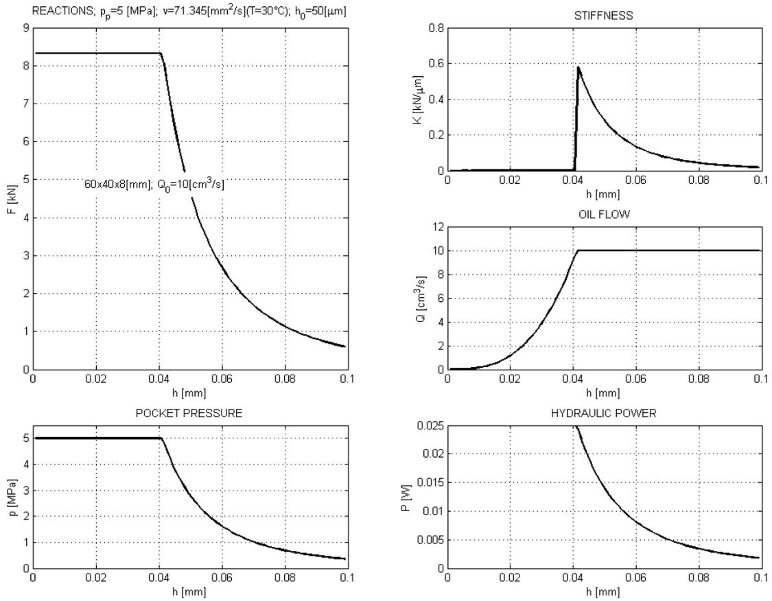
Fig. 4: Characteristics of the hydrostatic system with constant flow rate regulation
