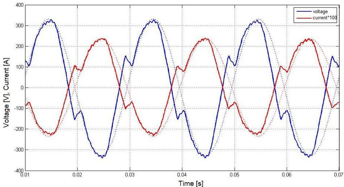
**Figure 6:** Output voltage and output current vs. time - load 350W @ 3000rpm
