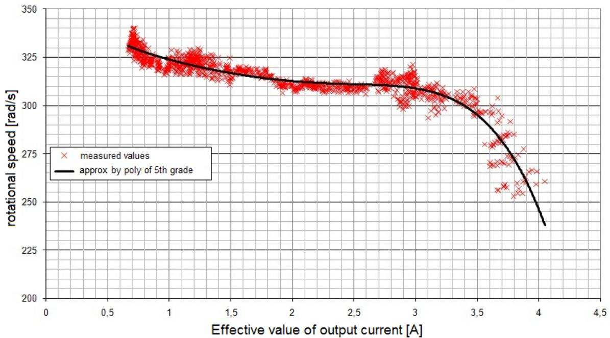
**Figure 2:** Rotational speed vs. effective output current - with original mechanical pendulum controller
