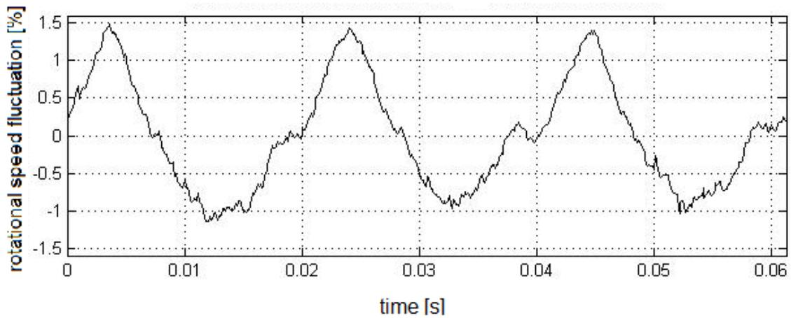
**Figure 3:** Rotational speed fluctuation of genset – load 670W @ 3000rpm
