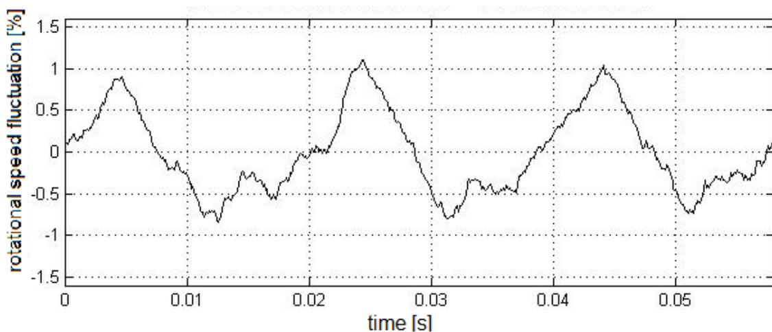
**Figure 4:** Rotational speed fluctuation of genset – load 270W @ 3000rpm
