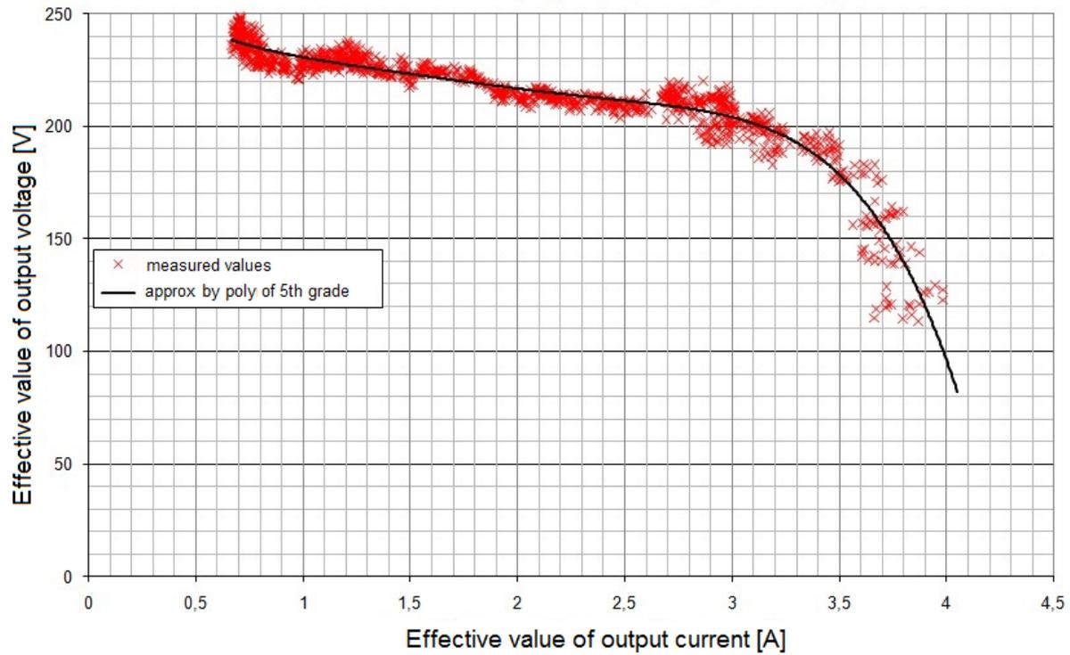
**Figure 1:** effective value of output voltage vs. effective output current - with original mechanical pendulum controller
