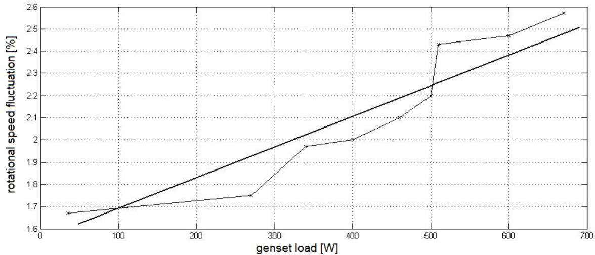
**Figure 5:** Rotational speed fluctuation vs. genset load @ 3000rpm
