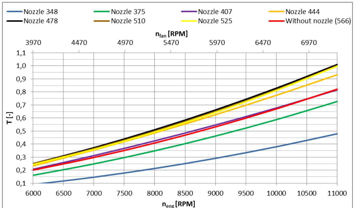
Fig. 19 – Dimensionless thrust, depending on the engine speed, resp. speed fan (chosen nozzle number corresponds to its diameter)
