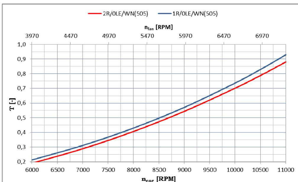
Fig. 21 – Comparison of the use of one and two radiators
