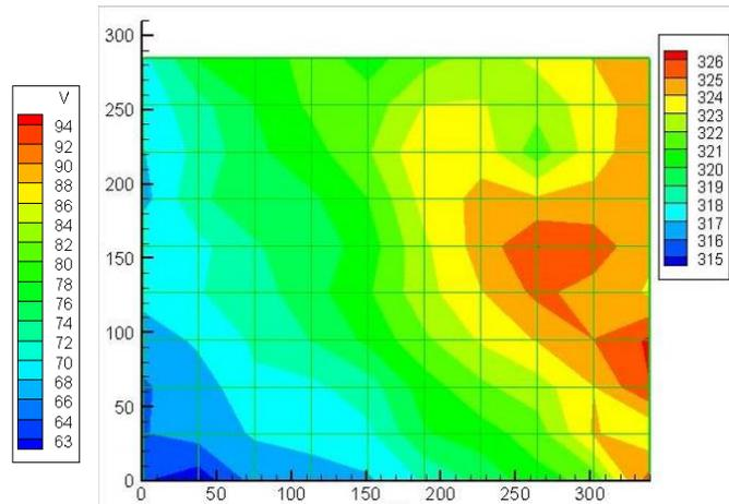
*Fig. 26 – Temperature field behind the radiator*
