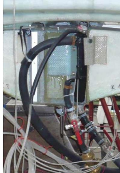
**Fig. 23** – A by-pass with a single radiator
