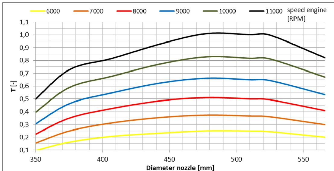
Fig. 20 – Dimensionless thrust at various engine speeds, depending on the diameter of the exit nozzle
