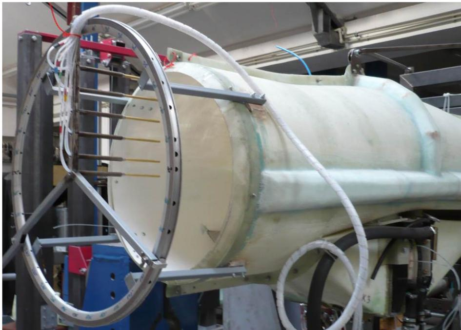
*Fig. 10 – Equipment for the measurement of pressure field in the output nozzle*
