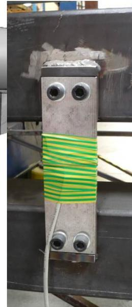
*Fig. 7 – Strips with strain gauges*
