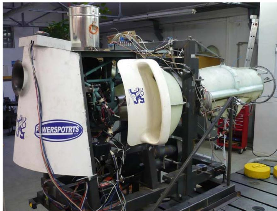
*Fig. 8 – Static test stand for the power unit in the laboratory*
