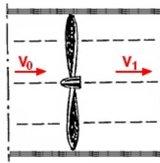
Fig. 2 – Propeller in a ring
