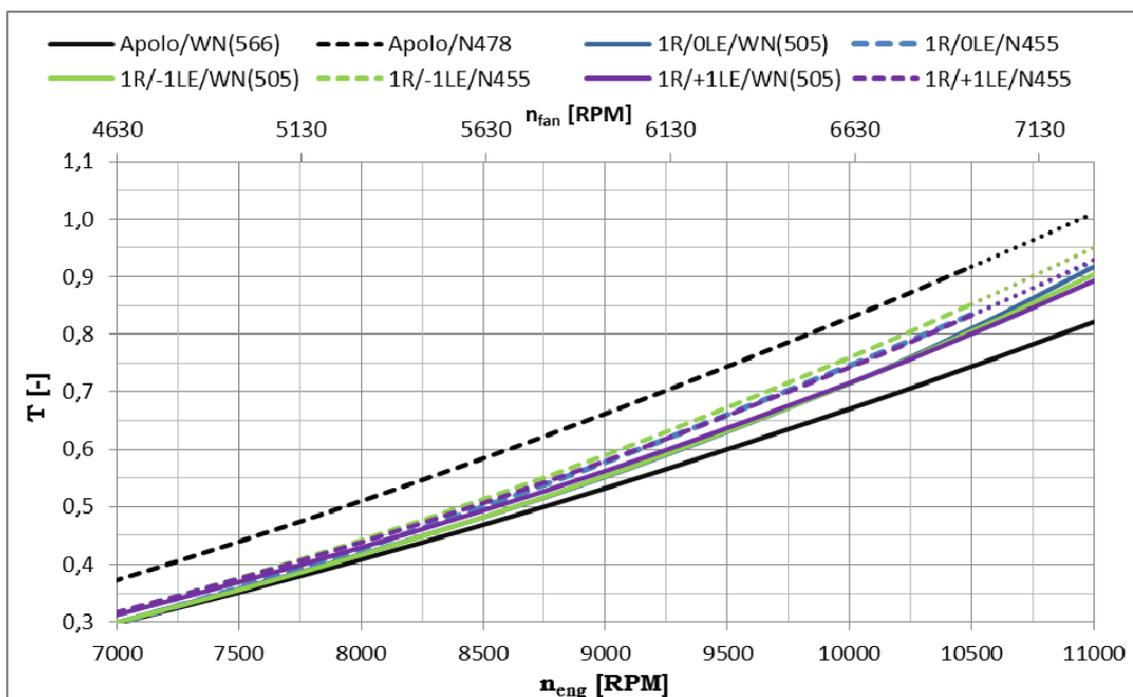
**Fig. 24** – Dimensionless thrust, depending on the engine speed, respectively fan speed for different configurations with one radiator
