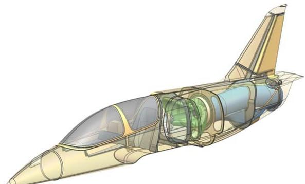
**Fig. 28** – Location of propulsion system in the fuselage
