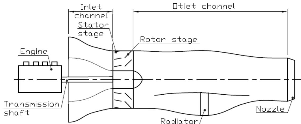
*Fig. 5 – Scheme propulsion unit*
