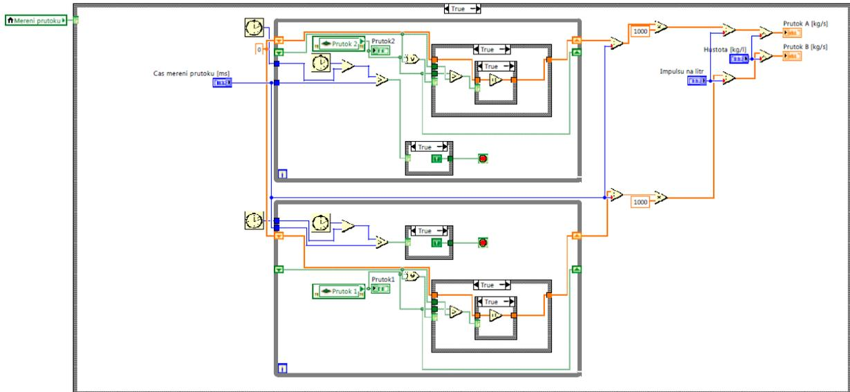
*Fig. 14 – Sample part of the block diagram - cooling water flow measurement*
