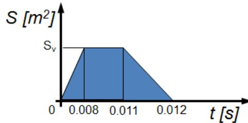
**Fig. 2.** Valve actuating function  $S(t)$
