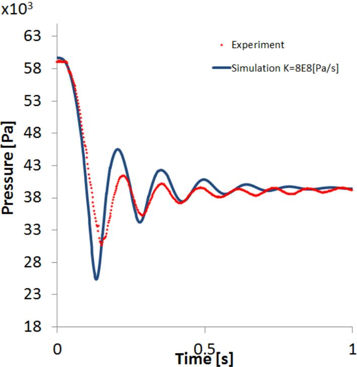
*Fig. 4. Pressure responses after almost instantaneously closed valve and simulation with three different constants  $k$ .*
