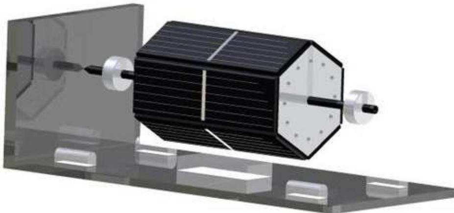
**Fig. 14.** Concept of Mendocino motor – motor is levitating above 2 neodymium magnets, which are replacing the bearings for no friction. Function of central neodymium magnet is described in Fig. 14. Because of opposite poles of neodymium magnets, motor is pushed towards the wall, making it stable in one position. There are several upgrades that can be made to improve its performance, such as adding more magnets and lamps around to create higher voltage on solar cells.
