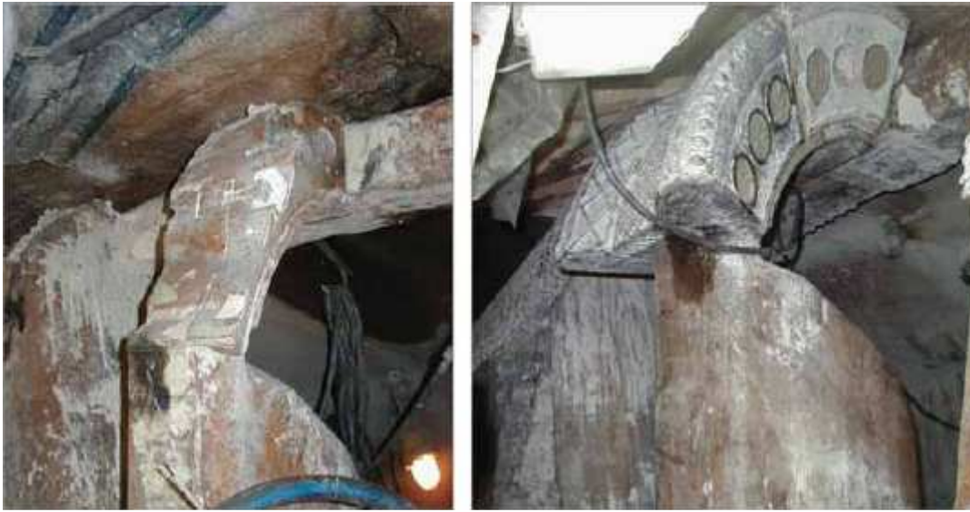
Fig. 9 The consequences of poor design of cutting head, the effects of abrasive wear
