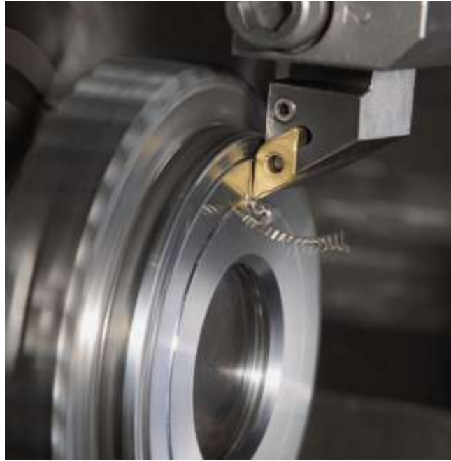
Fig. 1. Hard turning with the CB 7015 insert. [fot. Sandvik Coromant]
