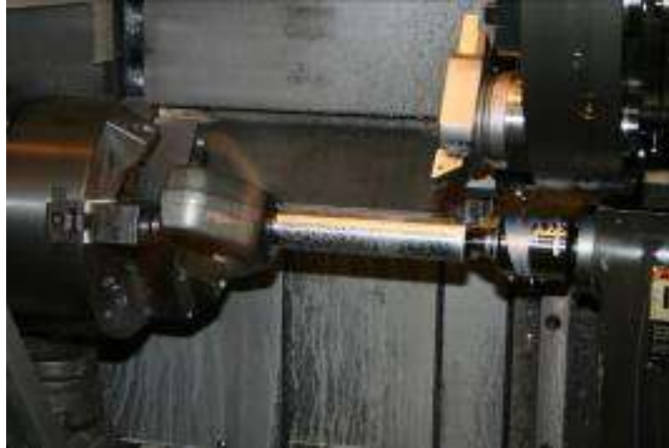
Fig. 4. Hard turning of the shaft on wet.
