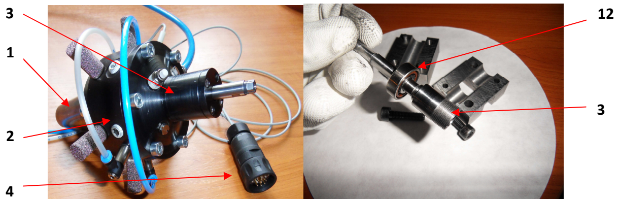
Fig. 1 Prototype of high speed milling spindle-left, assembly of spindle bearings- right
