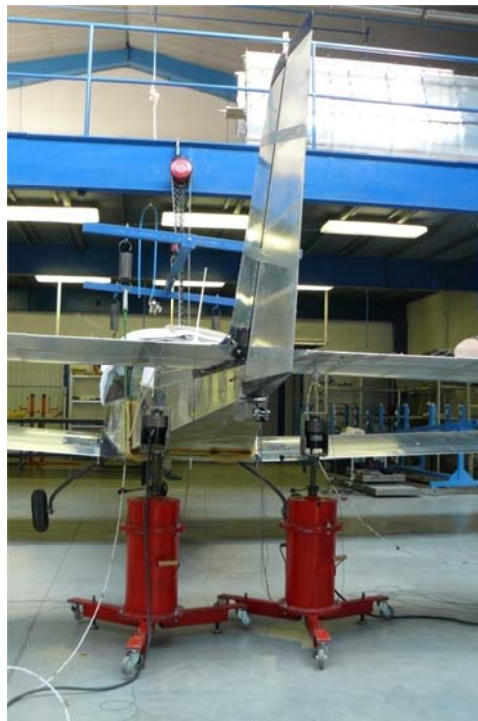
Fig. 5. Forcing of tail structure
