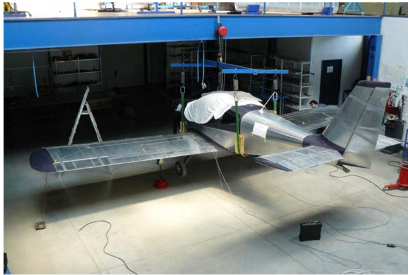
Fig. 4. Ground vibration test
