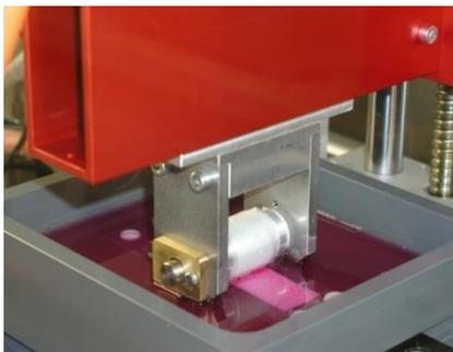
*Figure 1. Plowing experiment settings. Cartilaginous strip (2x20x60 mm) was glued to the bottom of the basin, which was filled with physiological solution that was kept at constant temperature 37°C. The steel indenter ( $\varnothing$  25 mm, high 40 mm) was lowered to the sample (force of 25 N, 50 N or 100 N was kept constant) and moved in the longitudinal axis of the sample with velocity of trapezoidal profile (10 mm/s peak value). Cyclic loading lasted 2 hours.*
