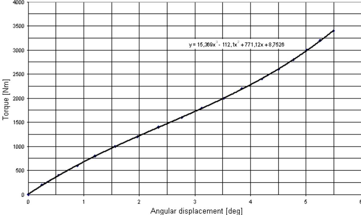
Fig. 8. Relation between torque and angular displacement.
