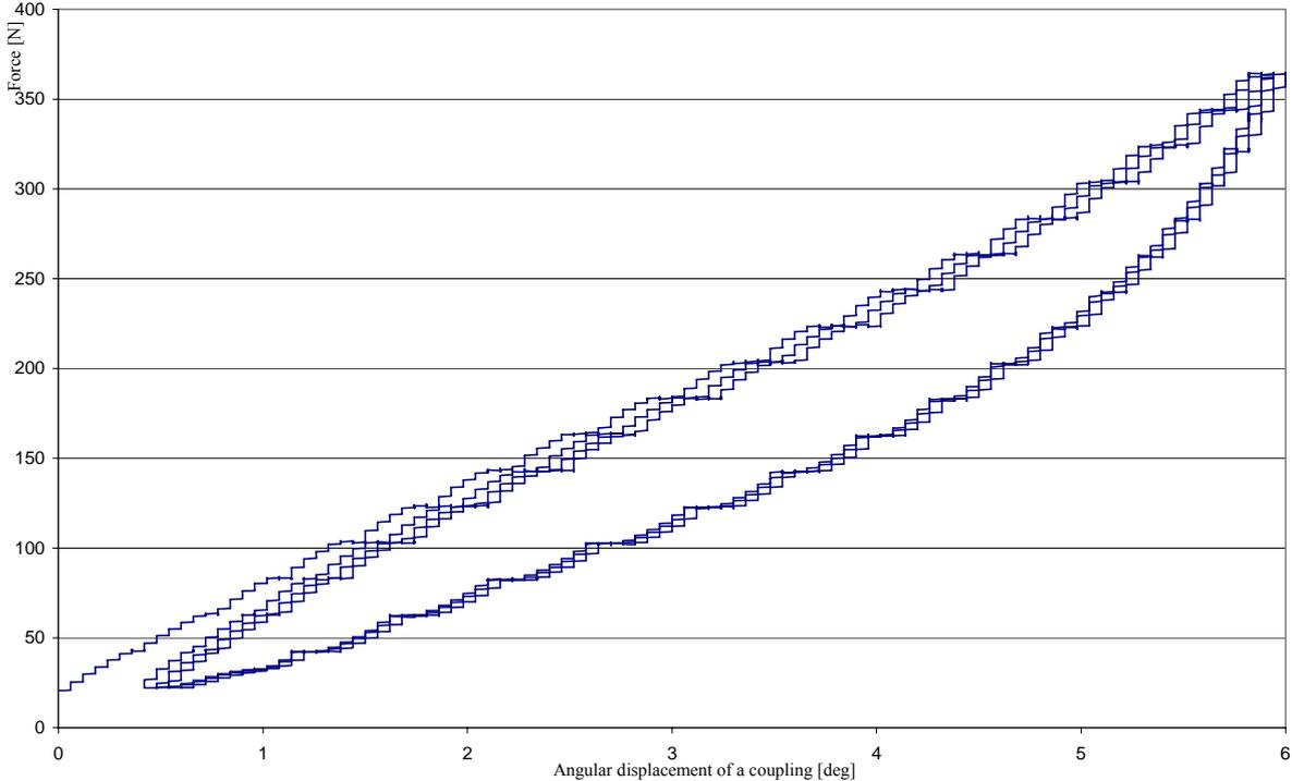
Fig. 7. Relation between torque and angular displacement during static torsion stiffness measurement.
