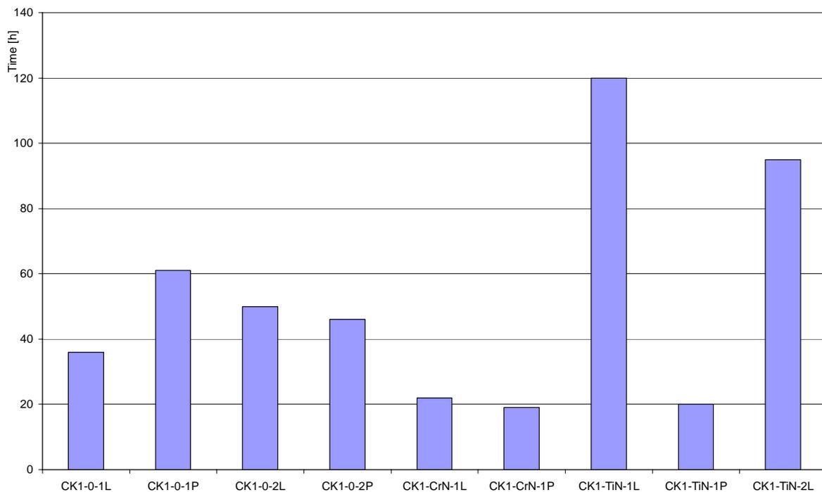
Fig. 16. Comparison of operating life of different coating types.
