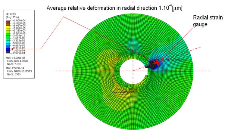
Fig. 14. Relative deformation on driving drum in FEM model.
