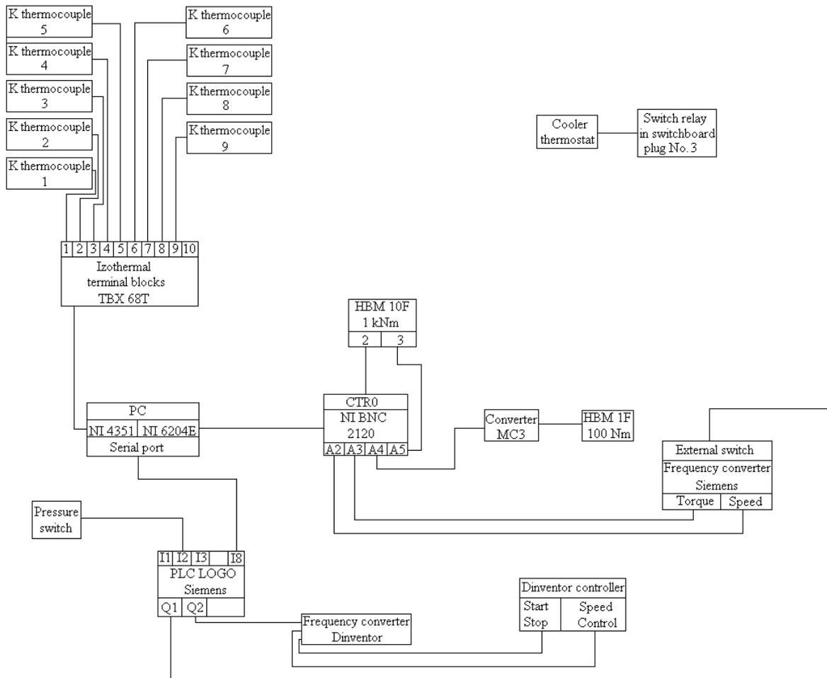
Fig. 3. Scheme of signal wiring.
