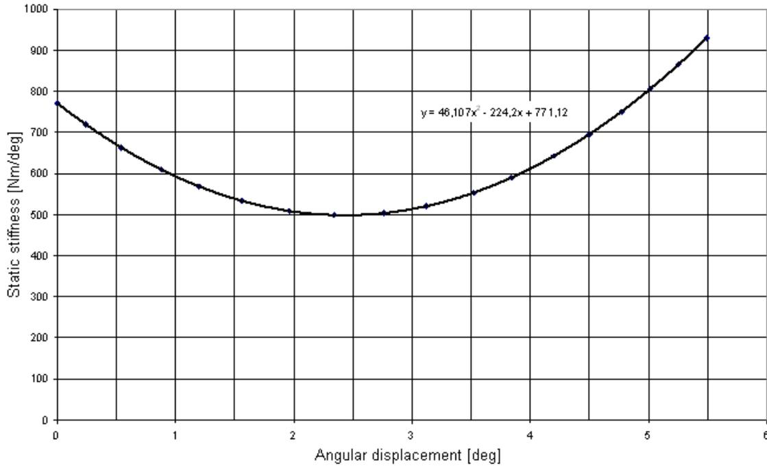
Fig. 9. Relation between static stiffness and angular displacement.
