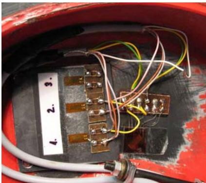
Fig. 13. Strain gauges on driving drum.
