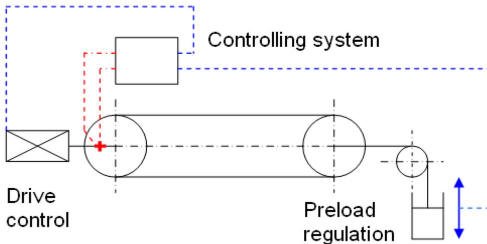
Fig. 15. Scheme of preload regulation.
