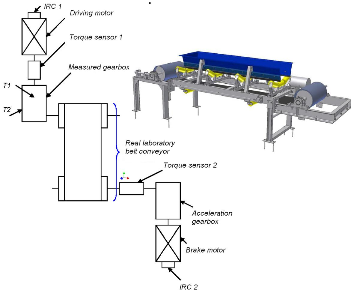
Fig. 11. Model of belt conveyor and scheme of test stand.
