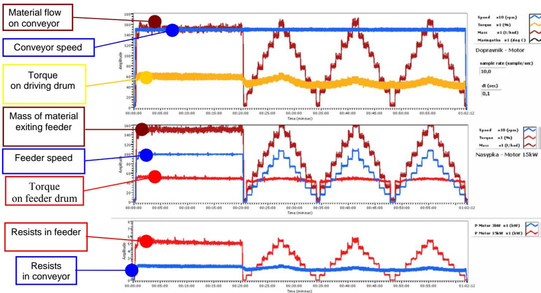
Fig. 12. Data measured during real run.
