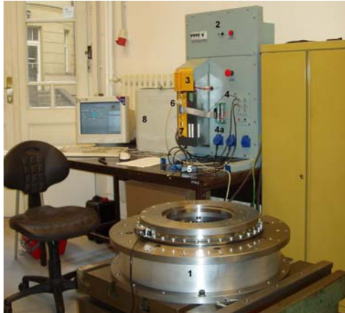
Fig. 8: Arrangement of experimental test bed with torque motor ROL 530881D
