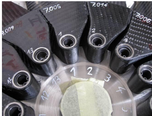
Fig. 4. Mounting of blades in the rotor disk.
