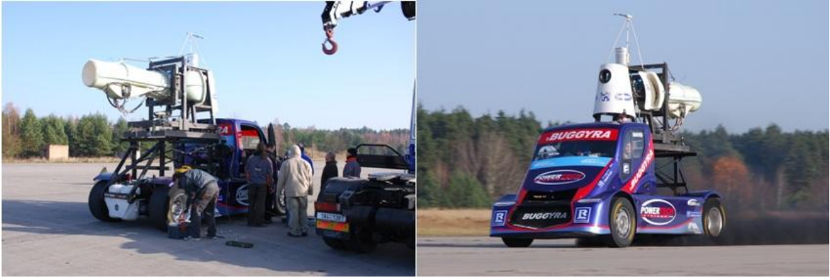
Fig. 14. Power unit mobile tests
