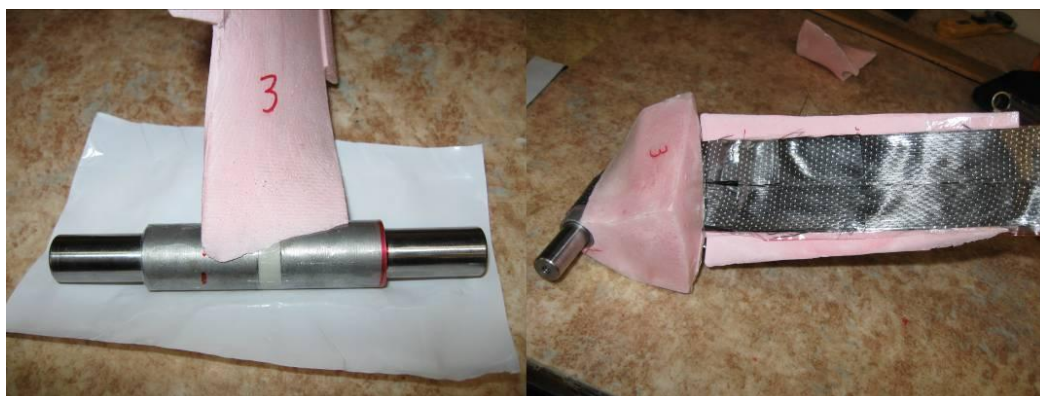
Fig. 6. The core of the leaf blade on the metal bushing and the addition of carbon flange and foot part foam core.
