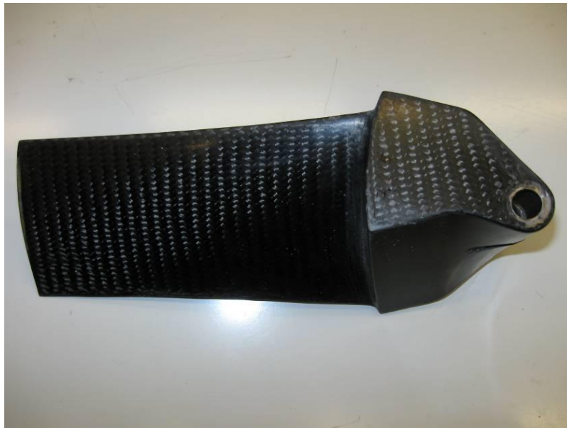
Fig. 8. Finished rotor blade after milling of rotor disk mounting groove.
