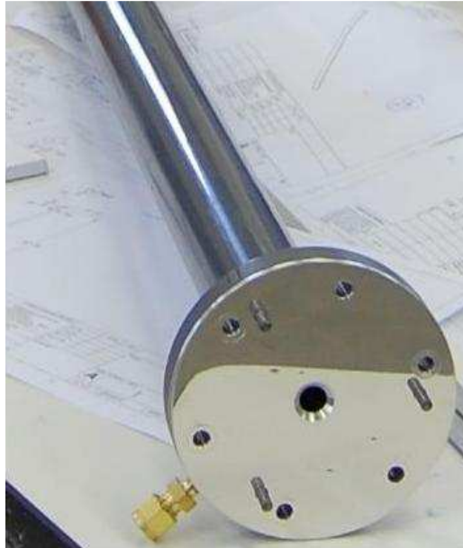
Figure 10. Manufactured orifice plate with a flange, PVC tube and a pressure tap attached to it
