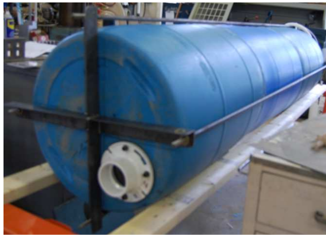
Figure 11. Manufactured barrel with inlet and outlet flanges
