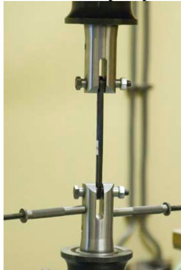
Fig. 9. Fatigue test of the fibre loops specimen with inner diameter d=10 mm
