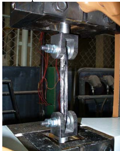
Fig. 6. Tensile test of fibre loop specimen
