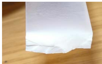
Fig. 19. Detail of the rupture of Veriflex ® shape memory polymer specimen, tensile test at 25° C.
