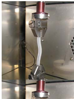
Fig. 2. Veriflex® specimen after DMA test – sliding of the specimen caused by low stiffness at high temperatures was observed.
