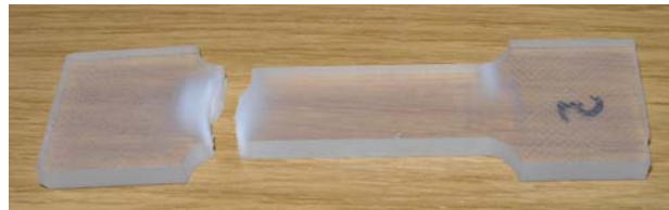
Fig. 18. Veriflex ® shape memory polymer specimen after tensile test at 25° C.
