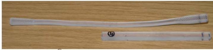
Fig. 21. Comparison of Veriflex ® specimen – the upper after tensile test at 70° C, the lower was never used for tests.
