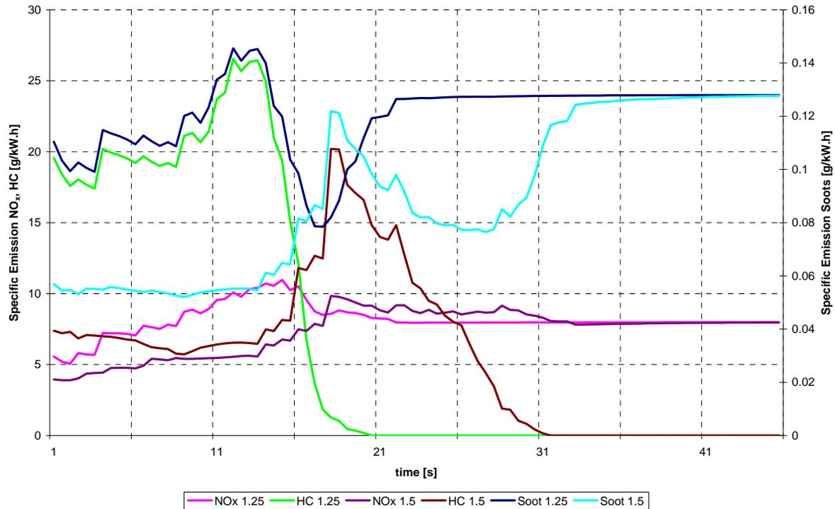
**Figure 5** – Specific brake emissions as a function of time at different limit values of relative A/F ratio during transient response to load change at constant engine speed
