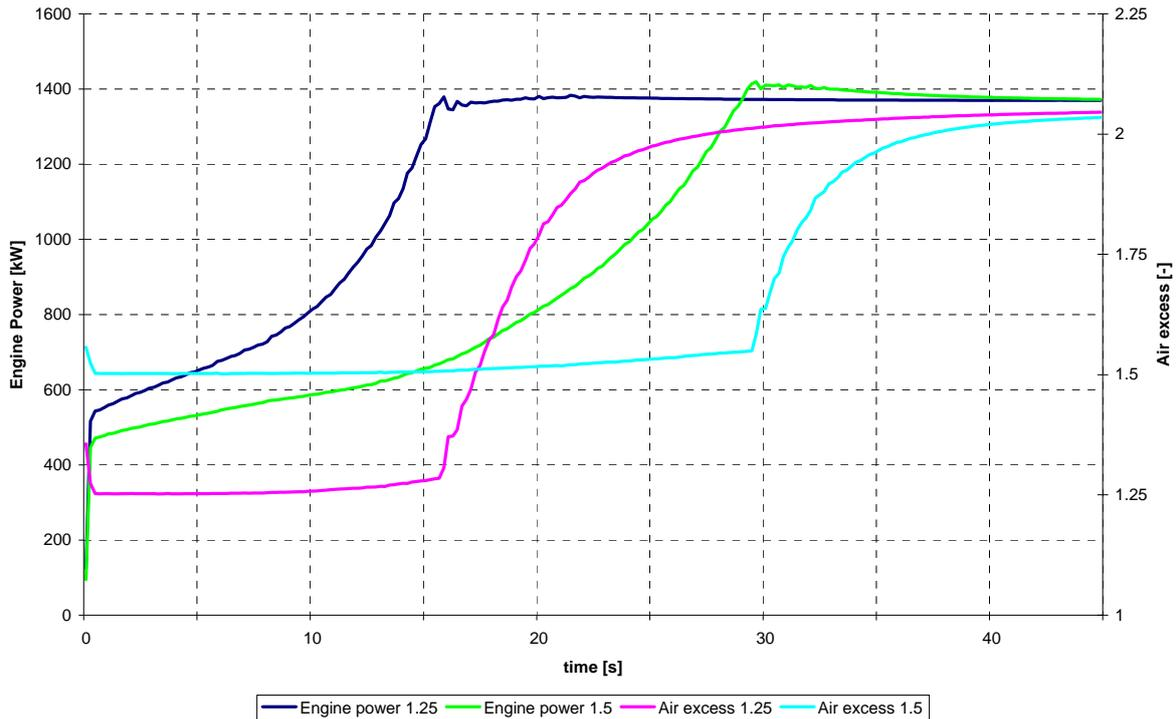
**Figure 3** – Engine power and relative A/F ration as a function of time at different limit values of relative A/F ratio during transient response to load change at constant engine speed
