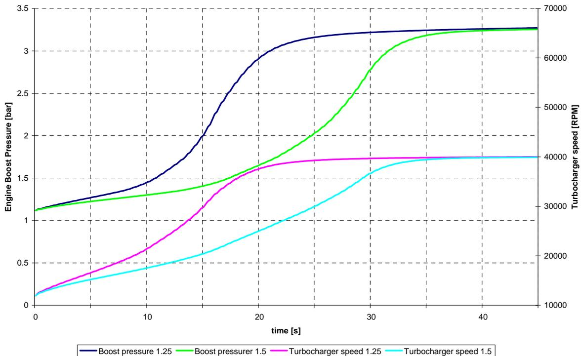
**Figure 4** – Pressure of intake air and turbocharger speed as a function of time at different limit values of relative A/F ratio during transient response to load change at constant engine speed
