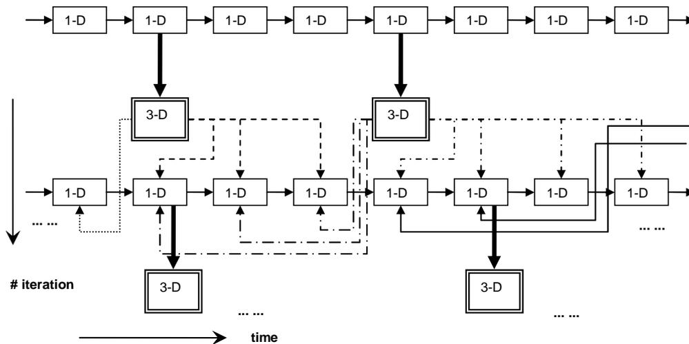
**Figure 1** Simulation scheme developed for transient operation simulation. Every rectangle refers schematically to a single engine cycle. The independent parallel 3-D simulations (assigned to 1-D previous run by bold arrows) provide for ROHR patterns and integral emissions per cycle. These results are stored in a library. The next 1-D run uses all previous results of 3-D by multidimensional interpolation in the database look-up tables between two most adjacent 3-D cycles.
