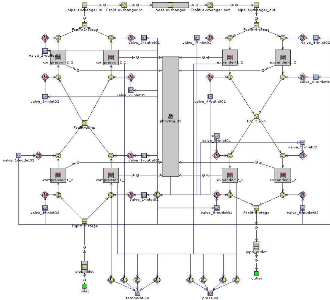
**Figure 6** GT Power model for simulation of the engine with double-acting stages 1, 2 – compressors and expanders
