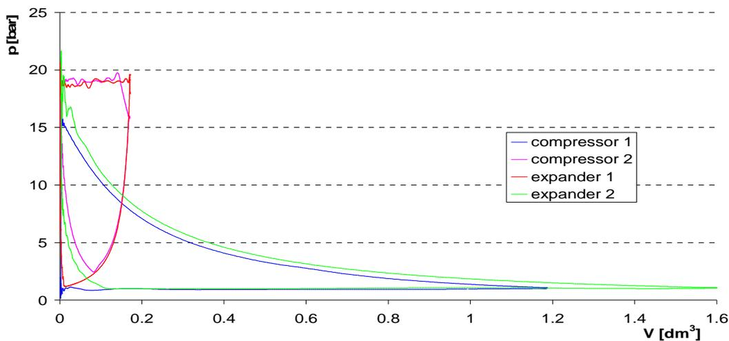
**Figure 8** Pressure diagrams of all positive displacement machines drawn against the volumes of individual machines. The useful work is produced mainly in the last machine 5 with slight contribution of 4. Compression takes place in 1 followed by some pressure increase in 2.
