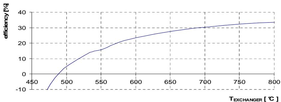
*Figure 11 Indicated efficiency in dependence on heat supply temperature*
