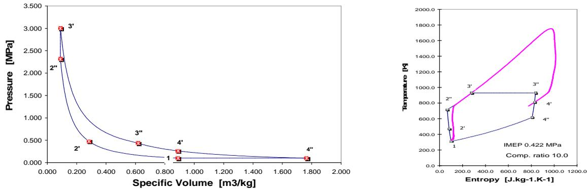
**Figure 1** p-V and T-s diagrams of five period cycle for IMEP of 0.422 MPa. Comparison to SI internal combustion engine of equivalent IMEP 0.85 MPa.
