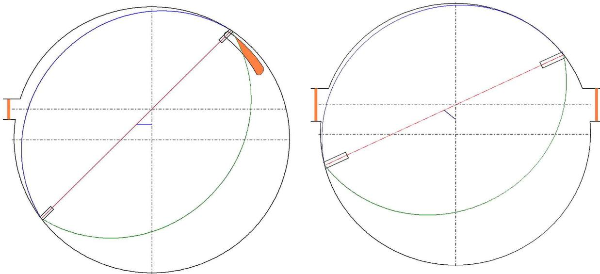
*Figure 4 Gas transfer ports: left combined radial and axial ones, right radial only*
