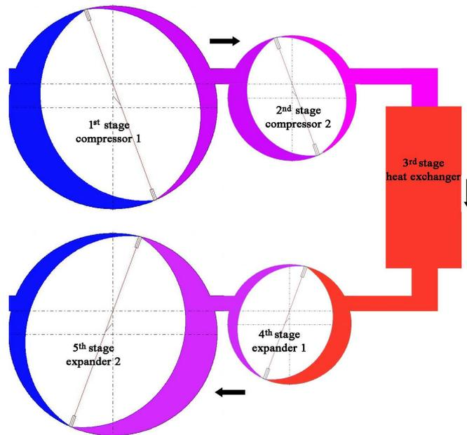
**Figure 5** The core of engine consisting of two stages creating a compressor, a heat exchanger and two stages creating an expander. Work is produced in the last stage and main compression takes place in the first one. The smaller stages between them realize gas exchange control mainly (Figure 9).
