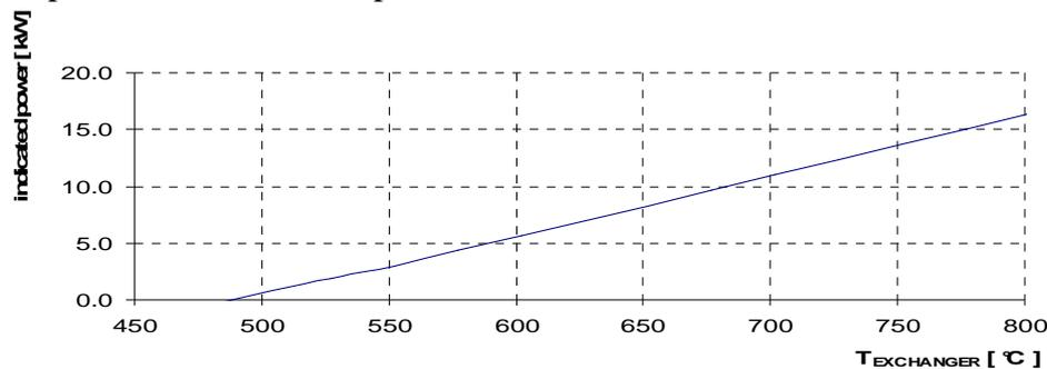
*Figure 10 Indicated power after optimization in dependence on heat supply temperature*
