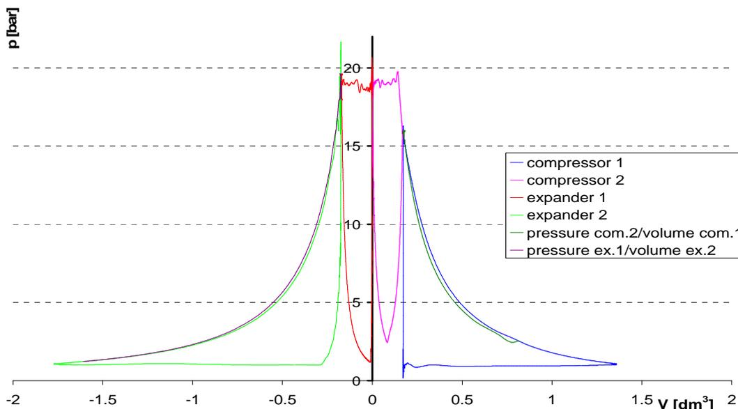
**Figure 9** Pressure diagrams of all positive displacement machines drawn against the cumulative volumes of compressing or expanding machines. The useful work is produced mainly in the last machine 5 with slight contribution of 4.
