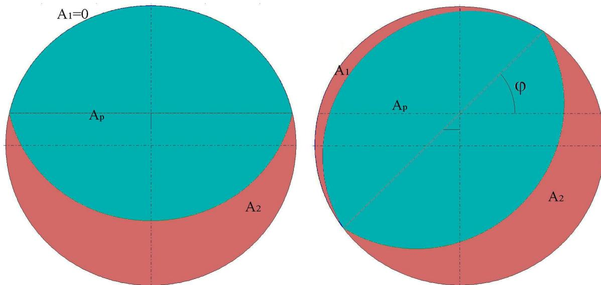
**Figure 3** Working spaces, at the right side in general position, at left the upper one in engine TDC and the other one in BDC
