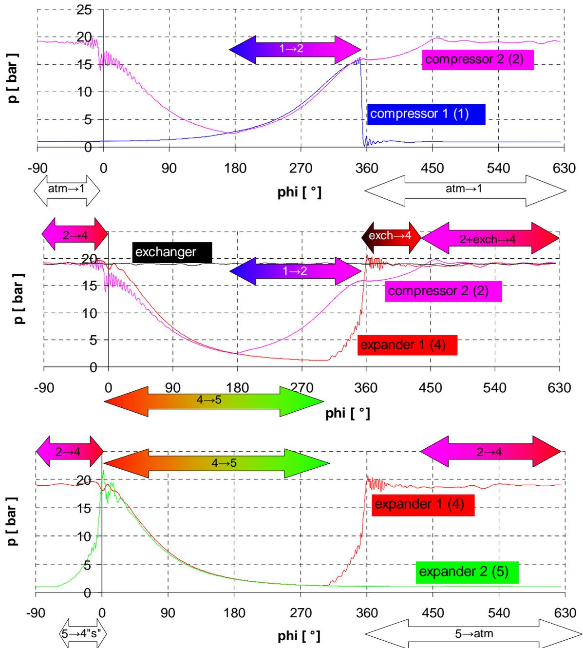
**Figure 7** Gas exchange timing and pressure traces for all compressors, a heat exchanger and expanders
