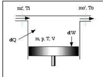
Figure 7: Scheme of generalized cell representing either a working space cell or heat exchanger cell [10].
