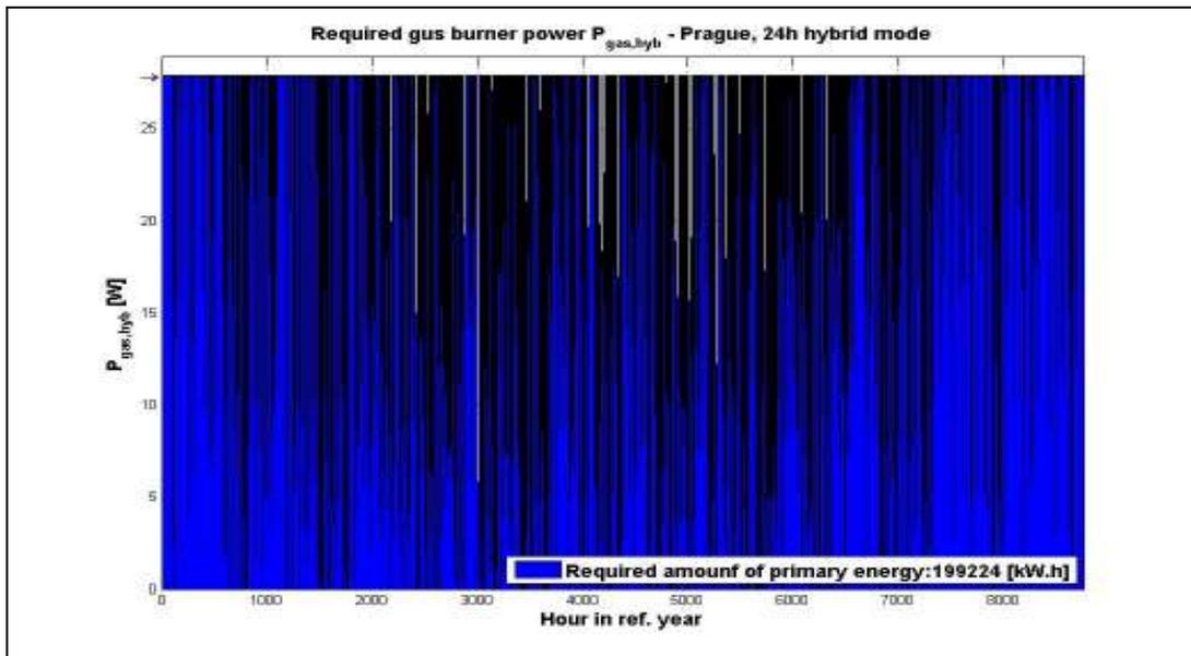
Figure 9: Gas burner power  $P_{gas,hyb.}$  as a function of solar radiation during the ref. year in Prague, 24h hybrid mode (gas burner is in operation if the  $P_{el.}$  of the HSSM is lower than  $10 \text{ kW}_e$ ). The maximum  $P_{gas,hyb.} = 27.87 \text{ kW}$  (marked by arrow) and the required amount of primary energy  $Q_{el,hyb.} = 199224 \text{ kW.h}$ .
