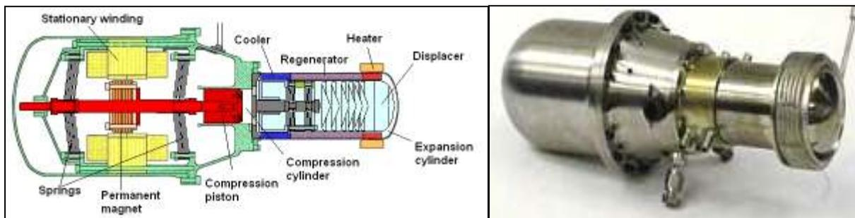
Figure 4: Scheme (left) and photo (right) of current Free-piston Stirling engine manufactured by Infinia - Stirling Technology Copany [7].
