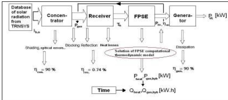
Figure 5: Schematic diagram of HSSM micro-cogeneration unit computational model solved in MATLAB.
