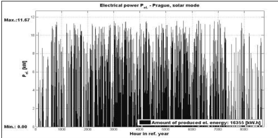
Figure 8: Electric power  $P_{el.}$  as a function of solar radiation during the ref. year in Prague (solar mode). The maximum  $P_{el.} = 11.67 \text{ kW}$  and the amount of produced el. energy  $Q_{el.} = 16355 \text{ kW.h}$
