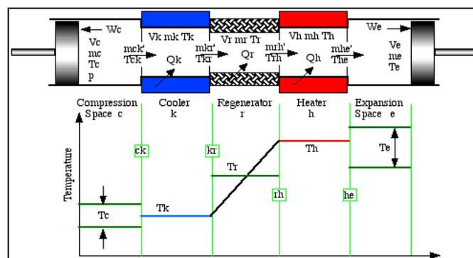
Figure 6: Scheme of FPSE Ideal Adiabatic Model (IAM) with temperature diagram [10].
