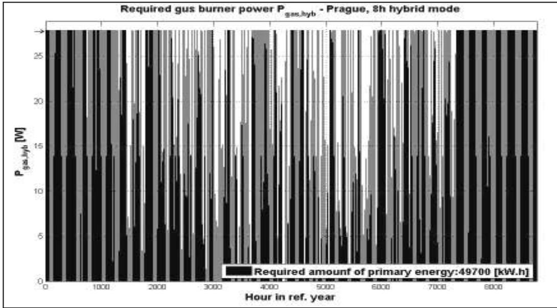
Figure 12: Gas burner power  $P_{gas,hyb}$  as a function of solar radiation during the ref. year in Prague, 8h hybrid mode (gas burner is in operation if the  $P_{el}$  of the HSSM is lower than  $10 \text{ kW}_e$  during the period from 8:00 until 16:00, only). The maximum  $P_{gas,hyb} = 27.87 \text{ kW}$  (marked by arrow) and the required amount of primary energy  $Q_{el,hyb} = 49700 \text{ kWh}$ .
