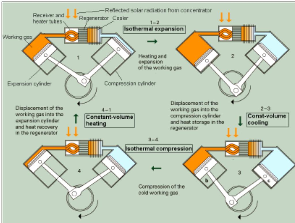
Figure 3: Description of four thermodynamic processes occurring in Stirling cycle during solar irradiation.
