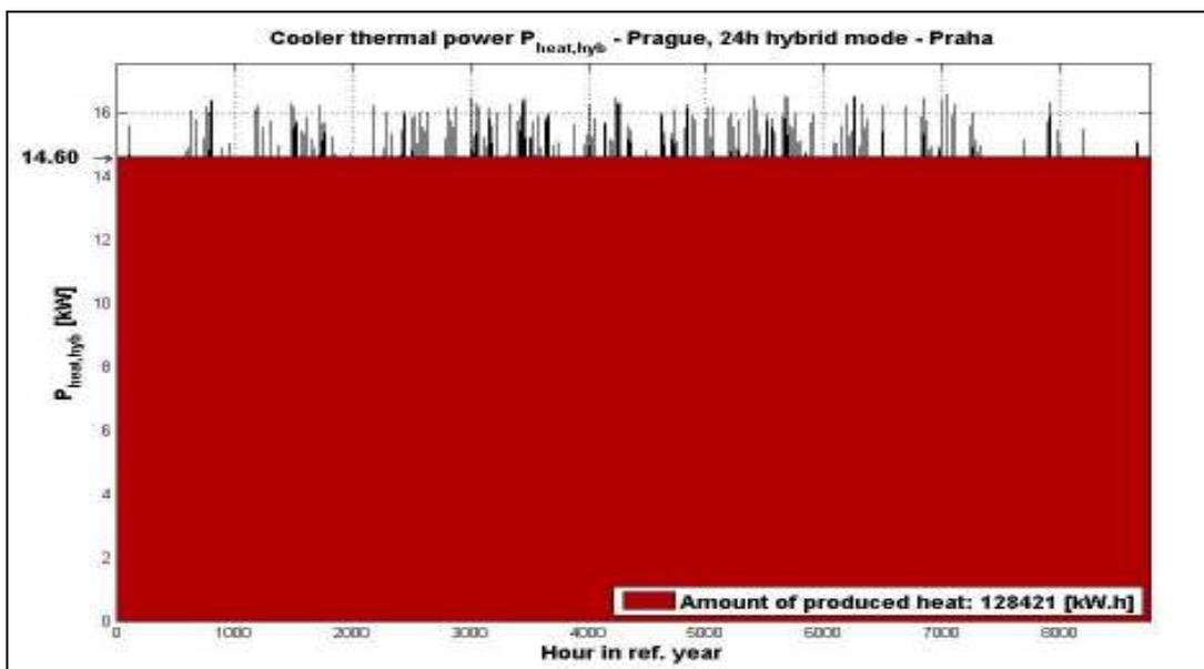
Figure 11: Cooler thermal power  $P_{heat,hyb}$ , as a function of solar radiation during the ref. year in Prague, 24h hybrid mode (gas burner is in operation if the  $P_{el}$  of the HSSM is lower than 10 kW<sub>e</sub>). The minimum  $P_{gas,hyb} = 14.6$  kW (marked by arrow) and the amount of produced heat  $Q_{heat,hyb} = 128421$  kW.h.
