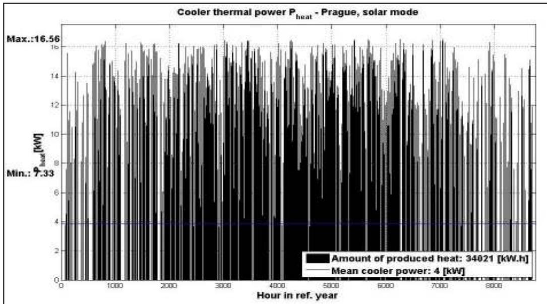
Figure 10: Cooler power  $P_{heat}$ , as a function of solar radiation, within the range of  $7.33 \div 16.56$  kW, during the ref. year in Prague (solar mode). The mean value of maximum  $P_{heat} = 4$  kW and the amount of produced heat  $Q_{heat} = 34021$  kW.h.
