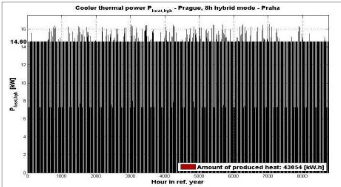
Figure 13: Cooler thermal power  $P_{heat,hyb}$  as a function of solar radiation during the ref. year in Prague, 8h hybrid mode (gas burner is in operation if the  $P_{el}$  of the HSSM is lower than  $10 \text{ kW}_e$  during the period from 8:00 until 16:00, only). The minimum  $P_{gas,hyb} = 14.6 \text{ kW}$  (marked by arrow) and the amount of produced heat  $Q_{heat,hyb} = 43054 \text{ kWh}$ .
