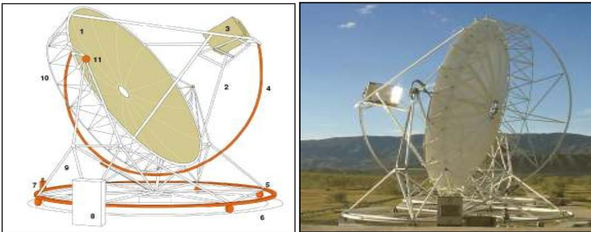
Figure 1: The scheme of Dish/Stirling system (left) - the Envirodish - and its current prototype (right) developed by German-Spain-France consortium [4] : 1) concentrator, 2) PCU support structure, 3) PCU, 4) elevation drive arc, 5) azimuth drive arc, 6) foundation, 7) azimuth drive, 8) switch case, 9) elevation bearing, 10) concentrator ring truss, 11) elevation bearing.
