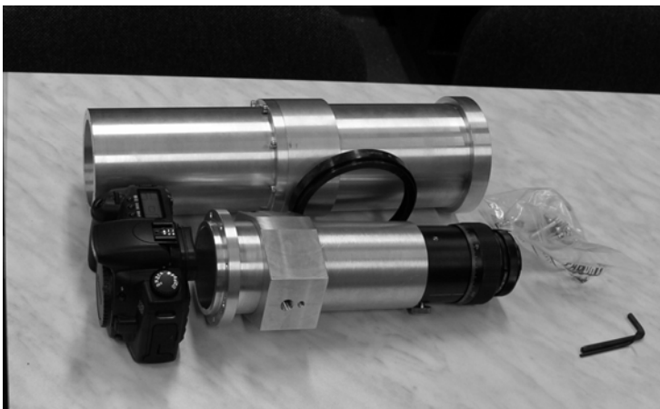
Pic. 3.5: Photo of manufactured Objective before it was painted.
