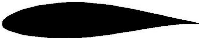
Figure 3: The Profile of the standard NACA 63-418 airfoil
