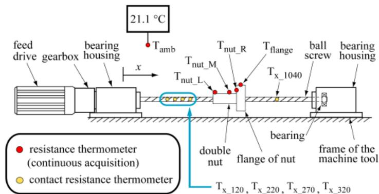
Figure 2.1: Scheme of test bed measurement with sensor locations
