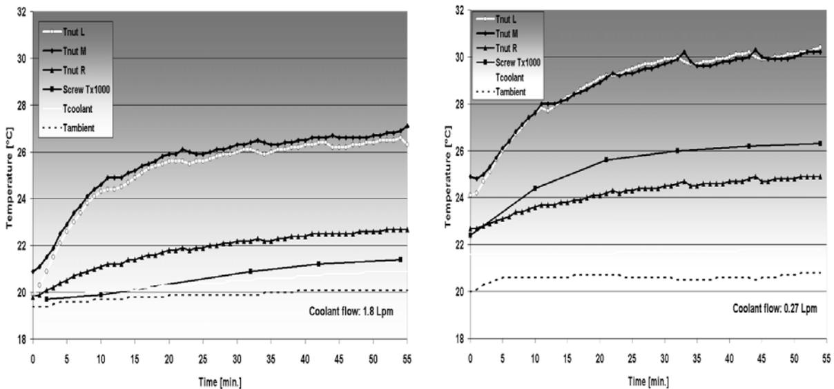
Figure 2.4: Chilled alternate; flow 1.8 Lpm on the left, 0.27 Lpm on the right
