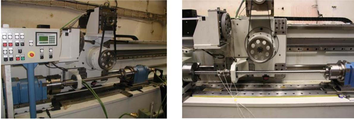
*Figure 2.2: Chilled and ordinary ball screws mounted at the test bed*
