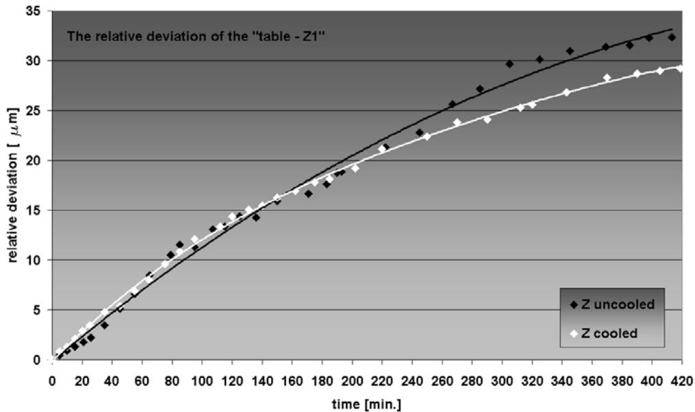
Figure 3.6: The Z1 point deviation compared with the table
