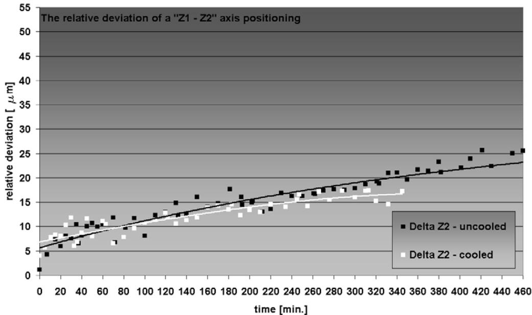
Figure 3.7: The Z2 point deviation compared with the Z1 point
