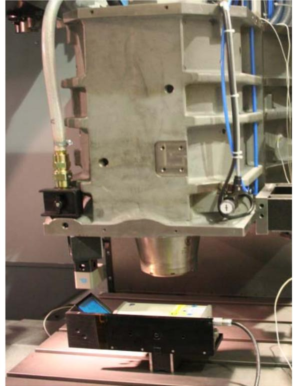
*Figure 3.2: Z axis positioning measurement*
