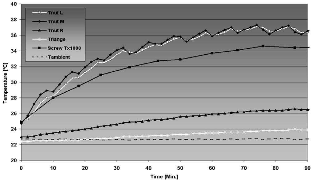
Figure 2.3: Measured data for revolution 800 rpm, loading force 3000 N and with the nut stroke 0.6 at the ordinary ball screw
