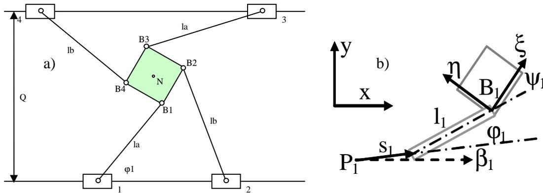
Fig. 5. : Design of Sliding Star (a), Design of one leg of Sliding Star (b)
