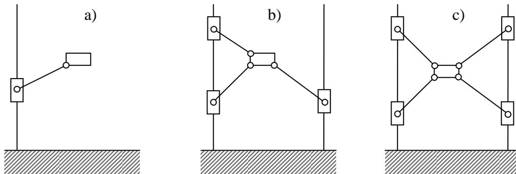
Fig. 1. : Serial (a), parallel (b) and redundant parallel (c) mechanism designs
