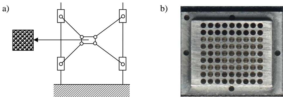
Fig. 4. : Non-redundant calibration design (a) and external calibration pin array (b)
