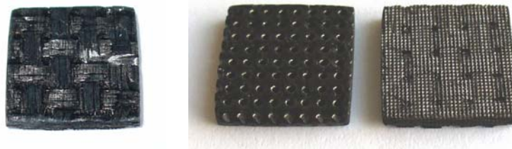
Fig.14 Textured carbon composites
