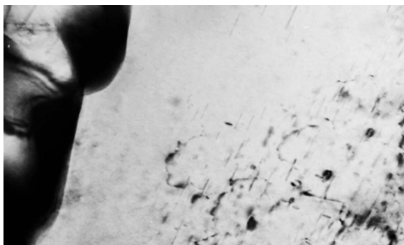
Fig. 8. Alloy B, aged for 5 hours, needle-shaped particles in [0001] \alpha -Mg direction in solid solution, TEM bright field image
